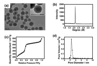
Fig. 2 Characterization of the structure and properties of HOTGTTGTimprinted MSNs. (a) TEM image (inset: a high-resolution image), (b) XRD pattern, (c) N<sub>2</sub> adsorption-desorption isotherms, and (d) pore size distribution.
