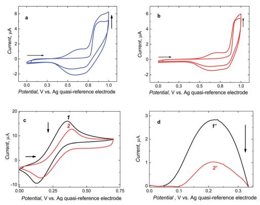
Fig. 2 Two-cycle potentiodynamic curves for deposition of (a) MIP (b) NIP films on 0.75 mm diameter Pt disk electrodes at a potential scan rate of 100 mV s<sup>-1</sup>. A DCM solution of (a) 0.1 mM CIL, (a) and (b) 0.3 mM FM1, (a) and (b) 0.3 mM CLM, and 0.1 M (TBA)ClO₄ was used for the electropolymerization. The (c) CV and (d) background corrected DPV curves for 10 mM ferrocene and 0.1 M (TBA)ClO<sub>4</sub> in DCM on (1, 1') the bare electrode, and (2, 2') the MIP-CIL film-coated electrode
