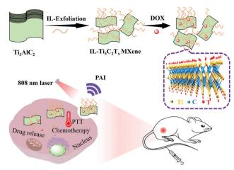
Scheme 1 Schematic illustration of the preparation of few-layer Ti<sub>3</sub>C<sub>2</sub>T<sub>x</sub> MXene nanosheets with high chemical stability using an IL-assist exfoliating method. The nanosheets can be used for photoacoustic imaging and the synergistic photothermal/chemotherapy of tumors.
