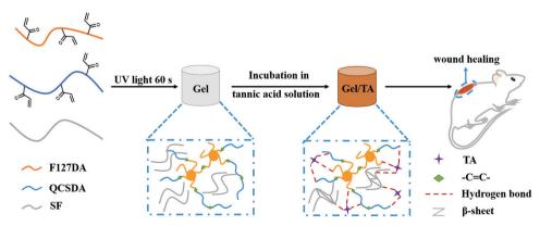
Scheme 1 A schematic diagram of Gel/TA hydrogel adhesive fabrication.
