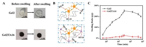
Fig. 2 The swelling behaviors of the hydrogels: (A) photos of the hydrogels Gel2 and Gel2TA16 before and after swelling; (B) schematic diagrams of the swelling principles for hydrogels Gel2 and Gel2TA16; and (C) the swelling ratios of the hydrogels Gel2 and Gel2TA16 (mean  $\pm$  SD, n=3).
