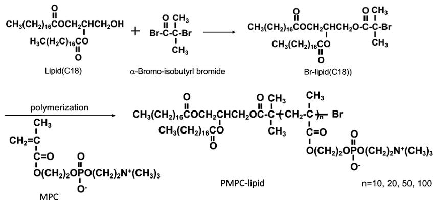
**Scheme 1** Schematic overview of the synthesis of Br-lipid initiator (C18). MPC was polymerized at Br-lipid(C18) by an ARGET-ATRP method with different degrees of polymerization. (C18); alkyl stearoyl chain, MPC; 2-methacryloyloxyethyl phosphorylcholine, ARGET-ATRP; activator regenerated by electron transfer-atom transfer radical polymerization.
