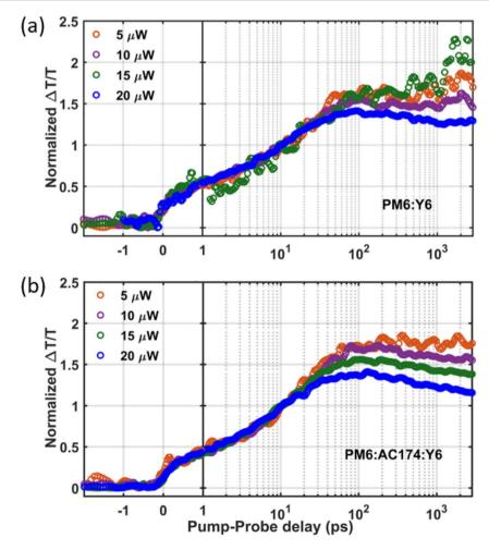
Fig. 4 Fluence dependent kinetics of the GSB signal for (a) PM6:Y6 and (b) PM6:AC174:Y6 films under an 800 nm excitation pump, intensity normalized at 10 ps.
