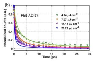
Fig. 3 (a) Integrated photoluminescence emission kinetics of PM6 and PM6:AC174 (5%) films. (b) Global fitting of fluence dependent decays for PM6:AC174 (5%) films.
