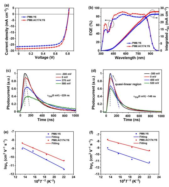
Fig. 2 (a) J-V curves and (b) EQE and integrated  $J_{SC}$  curves of optimized PM6:Y6 and PM6:AC174:Y6 devices. TPC curves of (c) PM6:Y6 and (d) PM6:AC174:Y6 devices at varied external bias voltages. Temperature dependence of hole mobility (e) and electron mobility (f) of PM6:Y6 and PM6:AC174:Y6 films in a  $\ln \mu$  vs.  $T^{-2}$  representation for quantitative analysis of the energy disorder.
