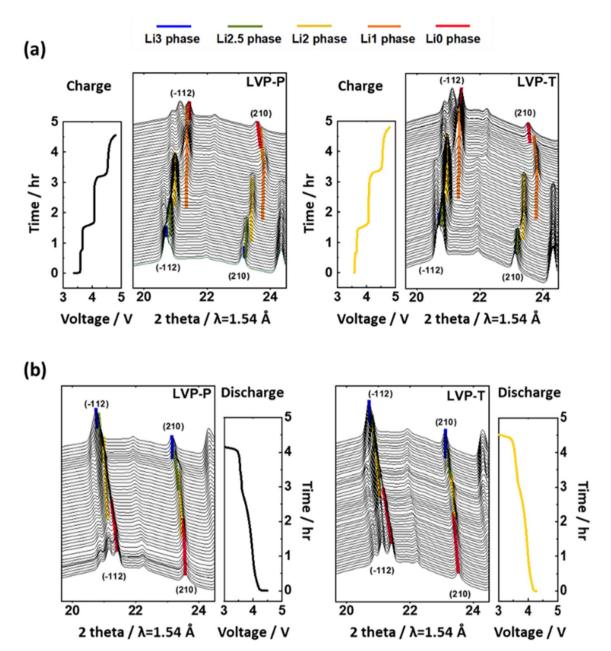
Fig. 4 In situ XRD patterns with time-voltage curve measured at 0.2C during the (a) 1st charge and (b) discharging process in the (-112), (210) planes of LVP-P (reproduced from ref. 44 with permission from The Royal Society of Chemistry) and LVP-T.
