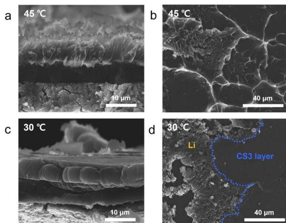
Fig. 4 (a and c) Cross-sectional and (b and d) top-view SEM images of the Li deposited CS3 composite anode plated to a capacity of  $3 \text{ mA h cm}^{-2}$  at (a and b)  $45 \text{ }^\circ\text{C}$  and (c and d)  $30 \text{ }^\circ\text{C}$ .
