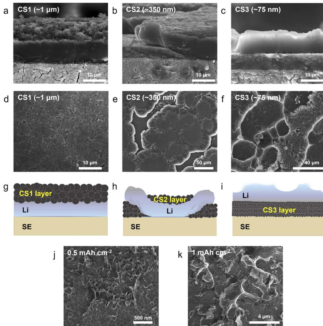
Fig. 2 (a–c) Cross-sectional and (d–f) top-view SEM images and (g–i) schematic illustrations of the Li in CS composite anodes deposited to a capacity of  $3 \text{ mA h cm}^{-2}$ . (a, d, and g) for CS1, (b, e, and h) for CS2, and (c, f, and i) for CS3. Top-view SEM images of Li deposits on the CS3 composite anode at capacities of (j)  $0.5$  and (k)  $1 \text{ mA h cm}^{-2}$ .
