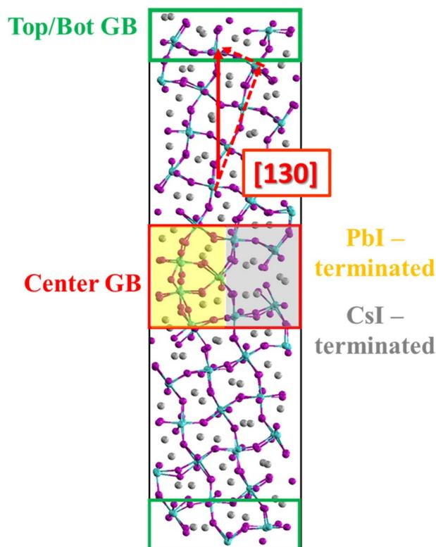
Fig. 1 Structural model of the  $\Sigma 5[130]$  GB of CsPbI<sub>3</sub> with the center GB and top/bot GB highlighted in red and green, respectively. PbI-terminated and CsI-terminated regions in the center GB are indicated by the yellow and gray regions, respectively.
