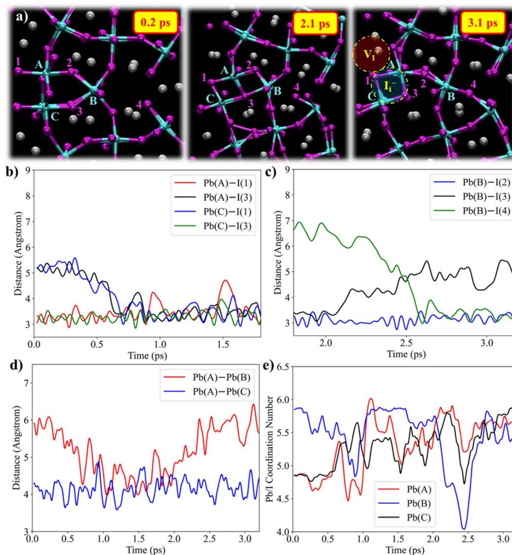
**Fig. 3** (a) Formation of an iodine Frenkel defect within the center GB. Letters and numbers consistently label the Pb and the I ions, respectively, which are relevant for the formation of the Frenkel defect. The Frenkel defect is highlighted in the right panel (b) and (c) give the time evolution of the Pb–I distances. (d) Time evolution of the Pb–Pb distances between the relevant Pb ions. (e) Time evolution of the Pb/I coordination number for each Pb ion.
