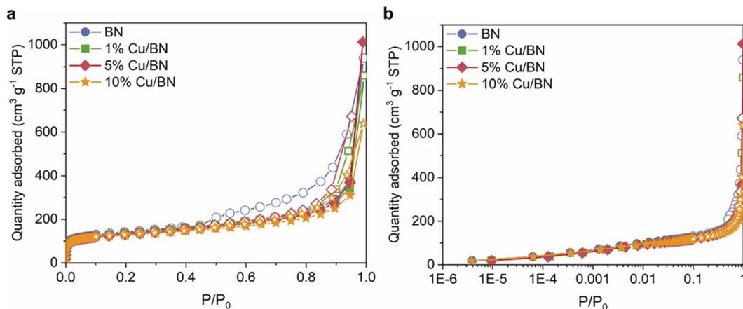
Fig. 5  $N_2$  sorption isotherms at 77 K for BN samples in (a) linear scale; (b) semi-log scale. Filled symbols: adsorption. Empty symbols: desorption.
