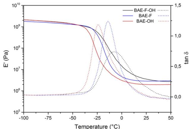
Fig. 3 Storage modulus (full curves) and  $\tan(\delta)$  (dotted curves) for BAE-F-OH (black curve), BAE-F (blue curve) and BAE-OH (red curve).
