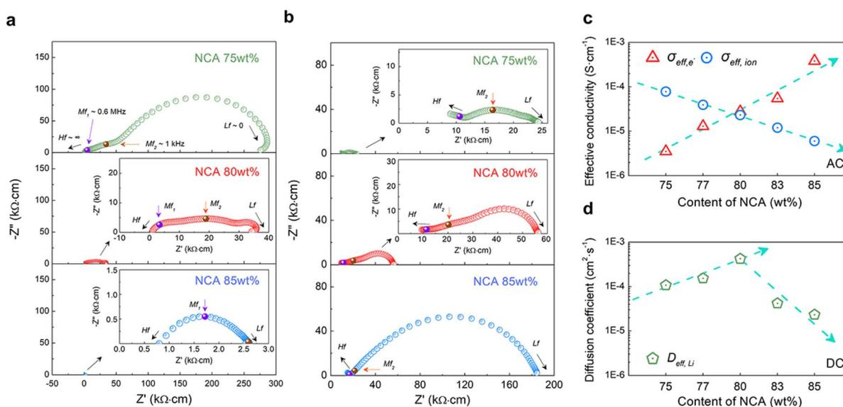
Fig. 4 Nyquist plots of (a) ion-blocking cells [SS||composite cathode||SS] and (b) electron-blocking cells [Li||LPSC||composite cathode||LPSC||Li] with 75 wt%, 80 wt%, and 85 wt% of NCA in composite cathodes. (c) Effective conductivity ( $\sigma_{\text{eff}}$ ) and (d) diffusion coefficients ( $D_{\text{eff},\text{Li}}$ ) results of the composite cathode extracted from EIS and DC polarization measurements as a function of NCA content from 75 wt% to 85 wt%.
