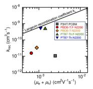
Fig. 8 Bimolecular recombination coefficient  $k_{\rm rec}$  determined by the EIS measurements compared with those calculated using the Langevin model expressed by eqn (15) (solid line). Different symbols represent the results of different devices as indicated by the legends in the graph.
