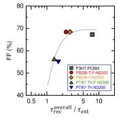
Fig. 4 FF  $versus~ au_{rec}^{overall}/ au_{ext}$  of the all-polymer blends and P3HT:PCBM blend solar cells. The dashed lines are drawn only to guide the eye. Different symbols represent the results of different devices as indicated by the legends in the graph.
