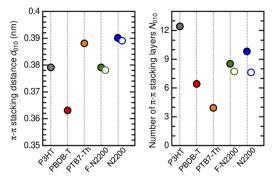
Fig. 6 Number of  $\pi-\pi$  stacking layers as obtained from the 1D diffraction profiles for every 2D GIWAXS pattern of the polymer donor and acceptor neat films. Open circles represent the results of the acceptor films processed with 0.5 wt% of DIO.
