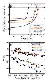
Fig. 1 (a) J-V characteristics of the devices under AM 1.5G (100 mW cm $^{-2}$ ) illumination: P3HT:PCBM (103 nm, black), PBDB-T:F-N2200 (94 nm, red), PBDB-T:N2200 (117 nm, orange), PTB7-Th:F-N2200 (106 nm, green), and PTB7-Th:N2200 (86 nm, blue). (b) Dependence of the FF of each device on the active layer thickness: P3HT:PCBM (squares), PBDB-T:F-N2200 (circles), PBDB-T:N2200 (diamonds), PTB7-Th:F-N2200 (triangles), and PTB7-Th:N2200 (inverted triangles).
