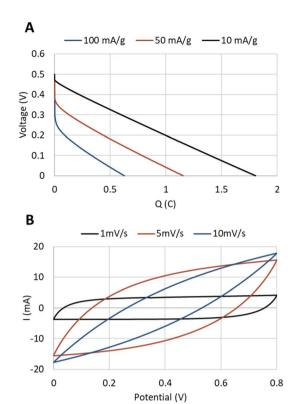
Fig. 4 Characteristics of the EDLC device. (A) Discharge at different discharge currents and (B) cyclic voltammetry at different scan rates.
