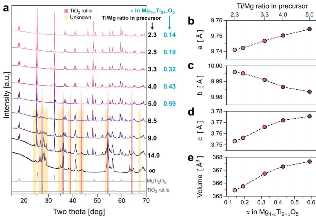
Fig. 3 (a) Series of XRD results of MTO synthesized from precursor with a  $\text{TiO}_2$  content greater than  $\text{Ti}/\text{Mg} = 2.3$ . Note that the remaining  $\text{TiO}_2$  rutile phase (indicated by the red box) appears in MTOs ( $\text{Ti}/\text{Mg} > 4.0$ ) from the excessive Ti in the precursor. (b–e) Relations between the unit-cell parameters and volume as a function of  $x$  in  $\text{Mg}_{1-x}\text{Ti}_{2+x}\text{O}_5$ .
