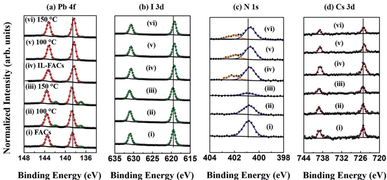
Fig. 3 High-resolution core level spectra of FAcS<sup>35</sup> and IL-FAcS thin films measured at RT, and at two different temperatures (100 °C and 150 °C) under UHV conditions (a) Pb 4f, (b) I 3d, (c) N 1s, and (d) Cs 3d. Spectra labelled (i, iv), (ii, v), and (iii, vi) correspond to the FAcS and IL-FAcS samples measured at RT, 100 °C, and 150 °C, respectively. For each condition, all spectra are normalized to the intensity of the Pb 4f<sub>7/2</sub> core level from Pb<sup>2+</sup>.
