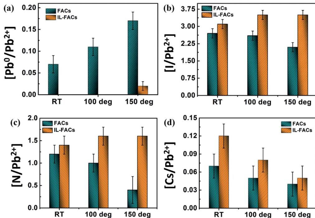
Fig. 4 (a–d) Elemental composition changes of the FACs and IL-FACs samples determined from XPS as a function of sample heating (a)  $Pb^0/Pb^{2+}$ , (b)  $I/Pb^{2+}$ , (c)  $N^*/Pb^{2+}$ , and (d)  $Cs/Pb^{2+}$  (\* the  $N/Pb^{2+}$  ratio presented in (c) includes only the N signal from the FA cation of the perovskite).
