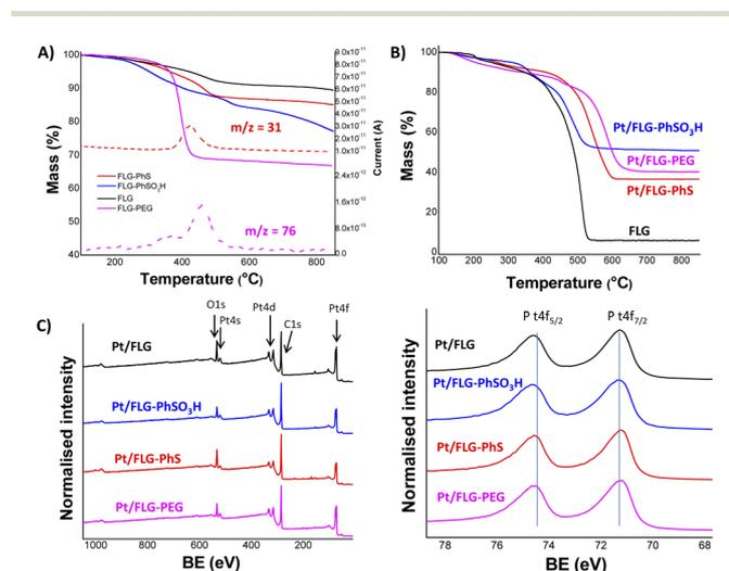
Fig. 1 Characterisation of functionalised graphene samples. (A) TGA-MS under N<sub>2</sub> of functionalised graphene samples. Phenyl and PEG fragments  $m/z = 76$  (C<sub>6</sub>H<sub>4</sub><sup>+</sup>) and  $m/z = 31$  (CH<sub>3</sub>O<sup>+</sup>), respectively. (B) TGA under air of platinum supported graphene samples. (C) XPS spectra of platinum supported graphene samples (left panel) and platinum Pt 4f component (right panel).
