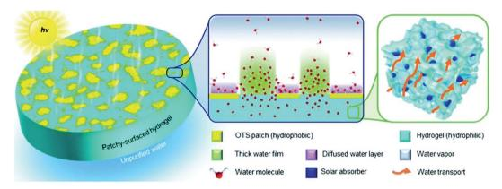
Fig. 11 Illustration of patchy-surface hydrogels (PSHs) for enhanced solar-driven evaporation. Reproduced with permission from ref. 104, copyright (2020) RSC.
