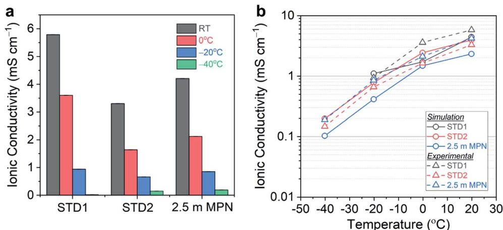
Fig. 2 (a) Total conductivity of the following electrolytes (STD1, STD2, and 2.5 m MPN) at room temperature, 0 °C, -20 °C, and -40 °C. (b) Total conductivity estimated using molecular dynamics simulations (O) and measured experimentally (Δ). The relative magnitudes among the three systems are consistent between MD and experiment, as are temperature trends.
