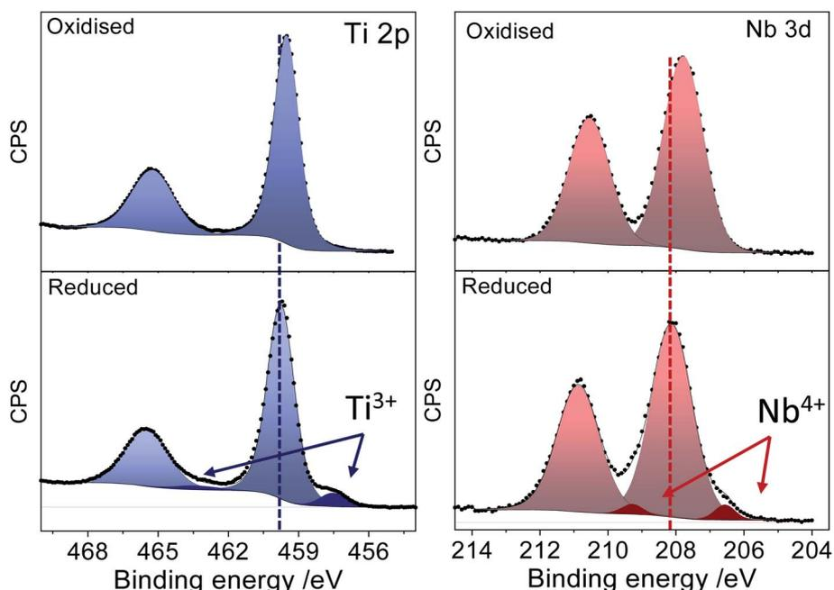
Fig. 3 XPS spectra of oxidised (upper panel) and reduced (lower panel) Nb doped TiO<sub>2</sub> in the Ti 2p and Nb 3d regions.
