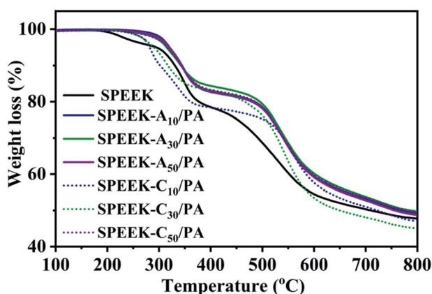
Fig. 2 TGA curves of SPEEK, SPEEK-A<sub>x</sub>/PA and SPEEK-C<sub>x</sub>/PA membranes.
