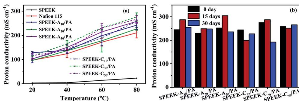
Fig. 5 (a) Proton conductivity vs. temperature at 100% R.H., and (b) proton conductivity (tested at 80 °C) after soaking in water at room temperature up to 30 days.
