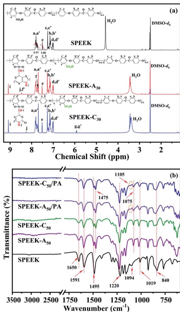
Fig. 1 (a)  $^1\text{H}$  NMR spectra of SPEEK, SPEEK-A<sub>30</sub> and SPEEK-C<sub>30</sub> in  $\text{DMSO}-d_6$ . (b) FTIR spectra of SPEEK, SPEEK-A<sub>50</sub> (or C<sub>50</sub>) and SPEEK-A<sub>50</sub> (or C<sub>50</sub>)/PA.
