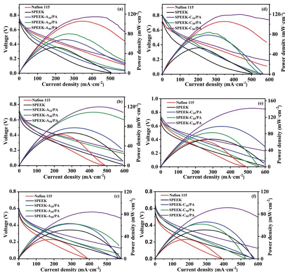
Fig. 6 Polarization and power density curves of SPEEK, SPEEK-A<sub>x</sub>/PA (a–c), SPEEK-C<sub>x</sub>/PA (d–f) and commercial Nafion 115 membranes with 1 M (a and d), 2 M (b and e), and 5 M (c and f) methanol as the fuel at 80 °C (methanol fuel with a flow rate of  $1 \text{ mL min}^{-1}$  and oxygen with a flow rate of  $30 \text{ mL min}^{-1}$ ).
