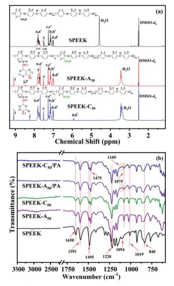
Fig. 1 (a)  $^{1}$ H NMR spectra of SPEEK, SPEEK-A $_{30}$  and SPEEK-C $_{30}$  in DMSO-d<sub>6</sub>. (b) FTIR spectra of SPEEK, SPEEK-A<sub>50</sub> (or C<sub>50</sub>) and SPEEK-A<sub>50</sub> (or C<sub>50</sub>)/PA.
