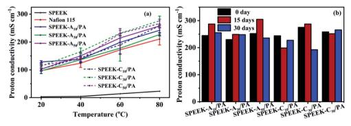
Fig. 5 (a) Proton conductivity vs. temperature at 100% R.H., and (b) proton conductivity (tested at 80  $^{\circ}$ C) after soaking in water at room temperature up to 30 days.
