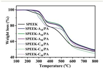
Fig. 2 TGA curves of SPEEK, SPEEK- $A_x/PA$  and SPEEK- $C_x/PA$  membranes.
