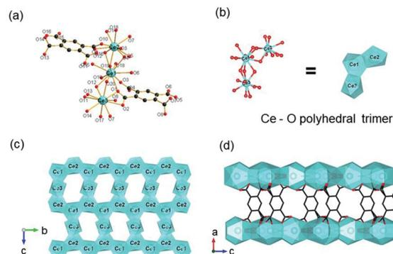
**Fig. 13** (a) The coordination environment of Ce(III) ions among CTH-15; (b) the structure of Ce–O polyhedral trimer *via* face-sharing; (c) the 2D structure of CTH-15 growing within the *b*–*c* plane; (d) the channel distribution of CTH-15 projected along the *b*-axis. Reproduced with permission from ref. 21. Copyright 2021, Elsevier Inc.
