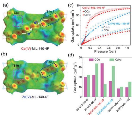
Fig. 19 The electrostatic potential distributions on the Hirshfeld surface of (a)  $Ce$ -MIL-140-4F and (b)  $Zr$ -MIL-140-4F (red-to-blue color indicates the high-to-low transition of electron density); (c) the  $CO_2$  and  $C_2H_2$  isotherms of  $Ce(IV)$ - and  $Zr(IV)$ -MIL-140-4F collected at 298 K; (d) the  $CO_2$  and  $C_2H_2$  uptakes of different MOF samples collected at 298 K. Reprinted with permission from ref. 30. Copyright 2021, WILEY-VCH Verlag GmbH.
