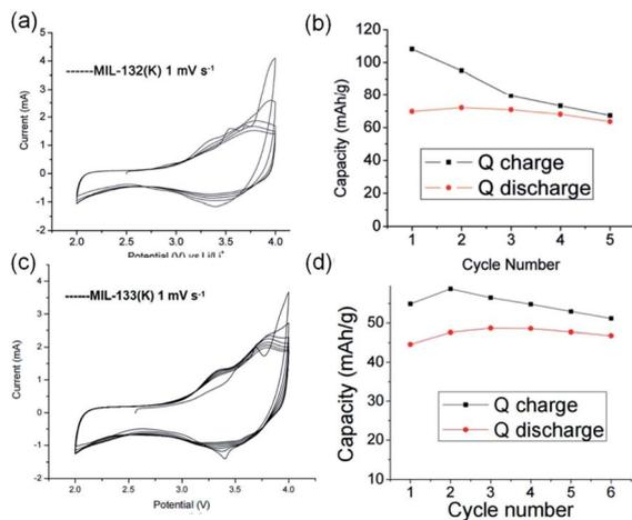
Fig. 21 (a) The solid-state cyclic voltammetry of MIL-132K between the 2 and 4 V vs.  $\text{Li}/\text{Li}^+$  at  $1 \text{ mV s}^{-1}$ ; (b) the charge and discharge capacity of MIL-132K within 5 cycles; (c) the solid-state cyclic voltammetry of MIL-133K between the 2 and 4 V vs.  $\text{Li}/\text{Li}^+$  at  $1 \text{ mV s}^{-1}$ ; (d) the charge and discharge capacity of MIL-133K within 6 cycles. Reprinted with permission from ref. 44. Copyright 2010, American Chemical Society.
