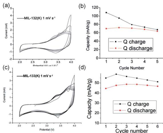
Fig. 21 (a) The solid-state cyclic voltammetry of MIL-132K between the 2 and 4 V vs. Li/Li<sup>+</sup> at 1 mV s<sup>-1</sup>; (b) the charge and discharge capacity of MIL-132K within 5 cycles; (c) the solid-state cyclic voltammetry of MIL-133K between the 2 and 4 V vs. Li/Li<sup>+</sup> at 1 mV s<sup>-1</sup>; (d) the charge and discharge capacity of MIL-133K within 6 cycles. Reprinted with permission from ref. 44. Copyright 2010, American Chemical Society.
