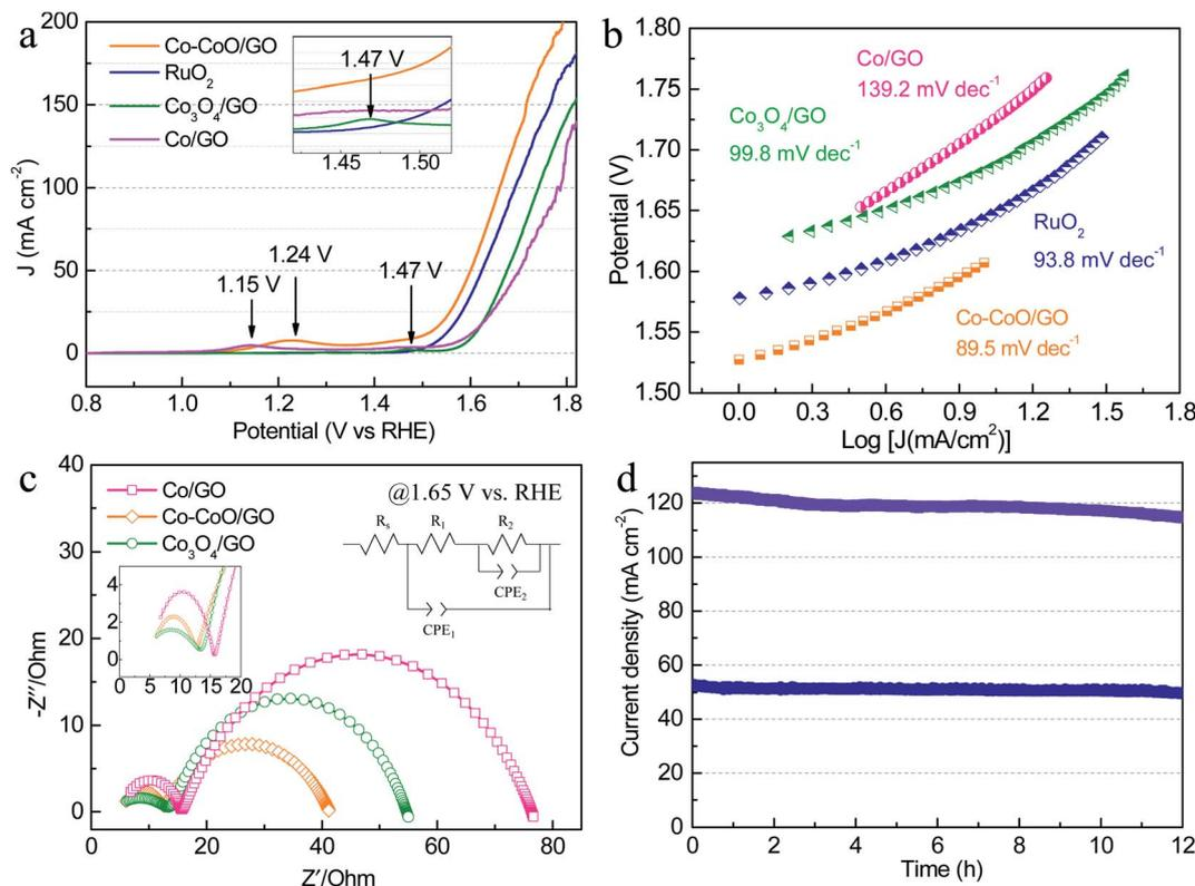
Fig. 2 (a) LSV curves and (b) corresponding Tafel slopes of Co/GO, Co–CoO/GO, Co<sub>3</sub>O<sub>4</sub>/GO and commercial RuO<sub>2</sub> in 1 M KOH. (c) EIS plots of Co/GO, Co–CoO/GO and Co<sub>3</sub>O<sub>4</sub>/GO at an overpotential of 420 mV. (d) The long-term amperometric (*i*–*t*) stability of Co–CoO/GO was measured at 1.63 and 1.71 V vs. RHE for 12 h.
