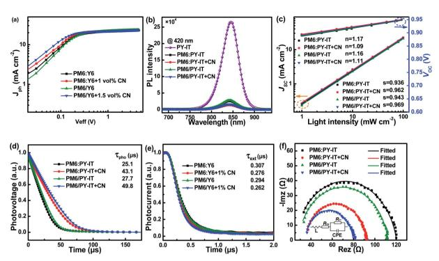
Fig. 3 (a)  $J_{\rm ph}-V_{\rm eff}$  curves of all-PSCs. (b) Photoluminescence spectra of the PY-IT film, and PM6:PY-IT and PM6/PY-IT blend films under 420 nm light excitation. (c)  $J_{\rm sc}-P_{\rm light}$  and  $V_{\rm oc}-P_{\rm light}$  curves of all-PSCs. (d) Transient photovoltage curves of all-PSCs. (e) Transient photocurrent curves of all-PSCs. (f) Nyquist plots and the equivalent circuit of all-PSCs.
