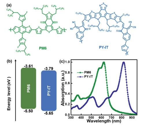
Fig. 1 (a) Chemical structures, (b) energy levels and (c) normalized absorption spectra of PM6 and PY-IT.
