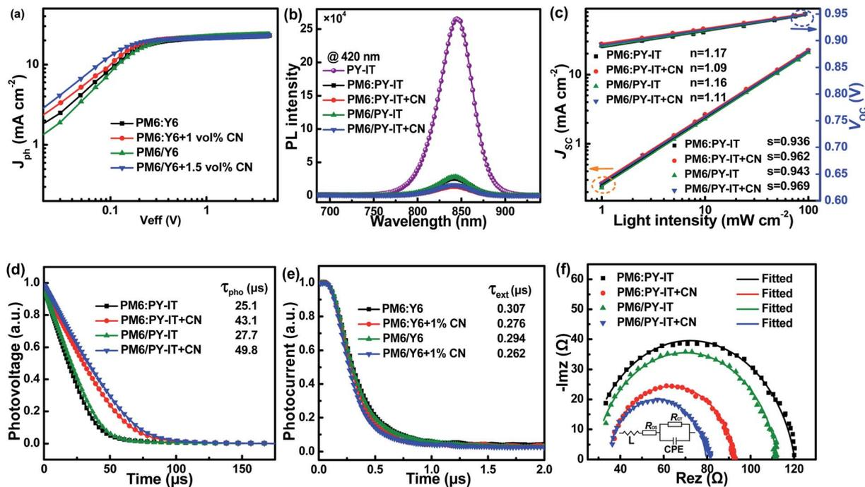
Fig. 3 (a)  $J_{\text{ph}}-V_{\text{eff}}$  curves of all-PSCs. (b) Photoluminescence spectra of the PY-IT film, and PM6:PY-IT and PM6/PY-IT blend films under 420 nm light excitation. (c)  $J_{\text{sc}}-P_{\text{light}}$  and  $V_{\text{oc}}-P_{\text{light}}$  curves of all-PSCs. (d) Transient photovoltage curves of all-PSCs. (e) Transient photocurrent curves of all-PSCs. (f) Nyquist plots and the equivalent circuit of all-PSCs.
