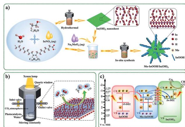
Scheme 1 (a) Synthesis diagrams of Mo modified  $\text{InOOH}/\text{In}(\text{OH})_3$ . (b) Schematic diagram of the  $\text{CO}_2$  photo-reaction system. (c) The proposed mechanism diagram of photocatalysis under visible-light irradiation ( $\lambda > 420 \text{ nm}$ ).
