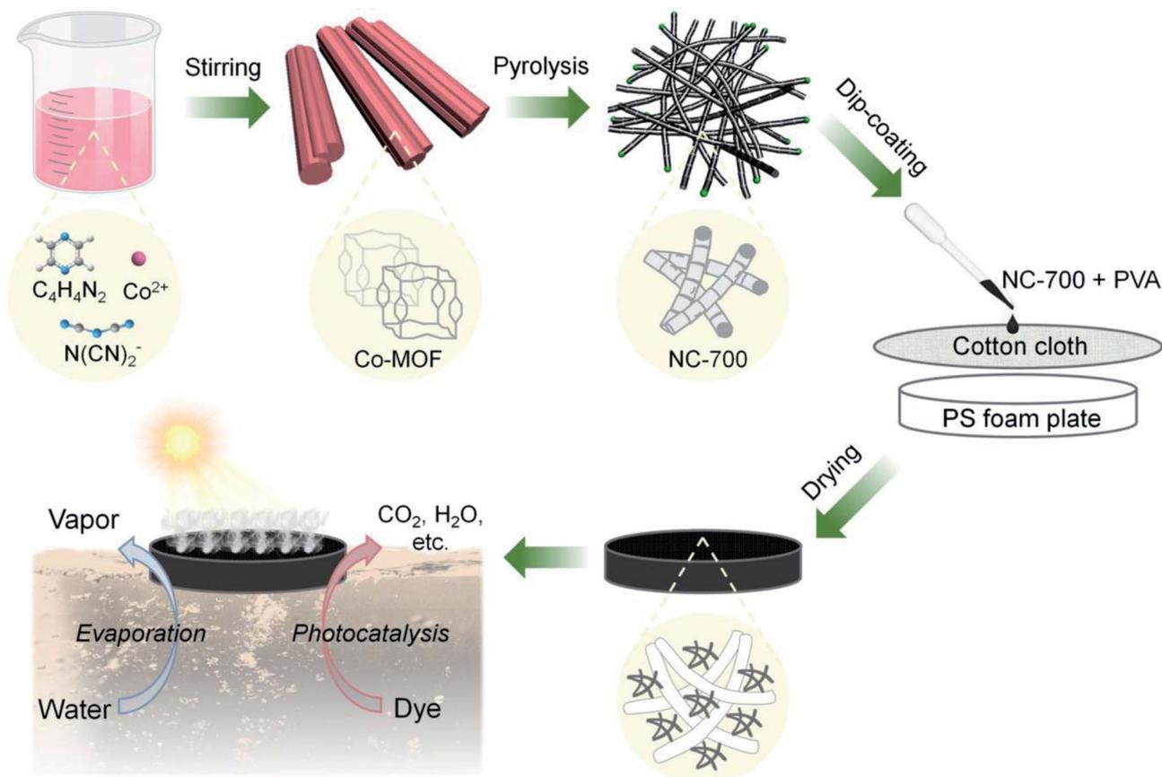
Fig. 1 Scheme of the fabrication of the bifunctional NC-*x* evaporator for interfacial solar-driven evaporation and the photocatalytic degradation of organic dyes (note: *x* stands for the calcination temperature, e.g., 700 °C; after coating, the PS foam plate was covered by the black NC-*x* evaporator).
