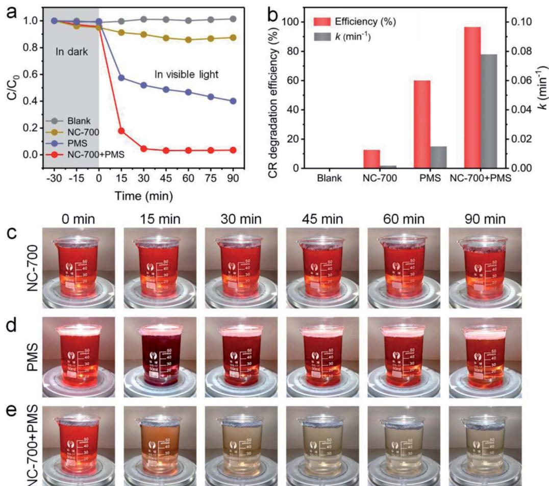
**Fig. 8** (a) The CR degradation efficiency within 90 min in different conditions. (b) The CR degradation efficiency and rate constant in different conditions. (c–e) Photographs of 100 ppm CR solution (75 mL) with NC-700 (30 mg), PMS (0.15 g L<sup>-1</sup>) and NC-700 + PMS under 1 sun irradiation.
