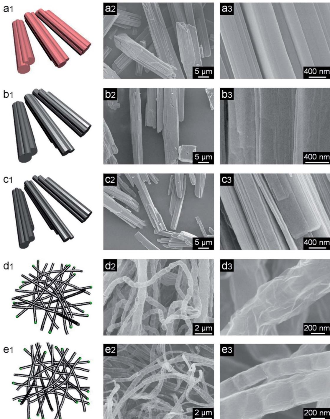
Fig. 2 Schemes (1<sup>st</sup> column) and SEM images (2<sup>nd</sup> and 3<sup>rd</sup> columns) of (a1–a3) Co-MOF, (b1–b3) NC-500, (c1–c3) NC-600, (d1–d3) NC-700, and (e1–e3) NC-800.
