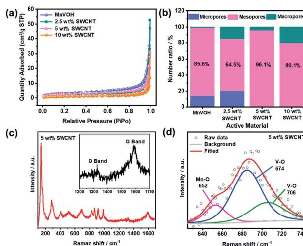
Fig. 3 BET analyses of MnVOH, 2.5 wt% SWCNTs, 5 wt% SWCNTs, and 10 wt% SWCNTs: (a) N<sub>2</sub> adsorption-desorption isotherms; (b) BET surface area. Raman spectrum: (c) 5 wt% SWCNTs (inset is the spectrum from 1200 to 1700 cm<sup>-1</sup>), and (d) partially fitted spectra to show the presence of the Mn-O bond.
