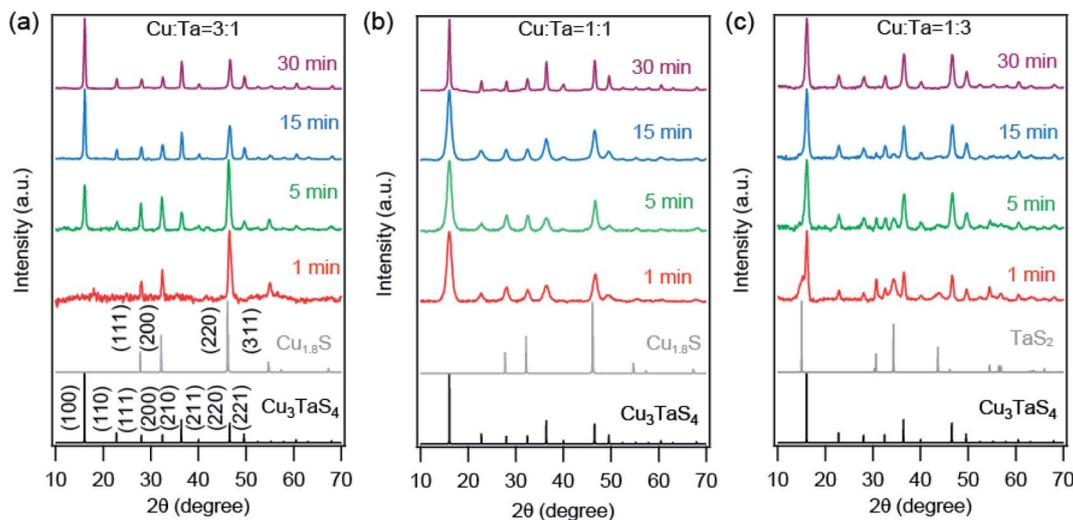
**Fig. 2** XRD patterns of synthesized Cu-Ta-S NCs for (a) Cu : Ta = 3 : 1, (b) Cu : Ta = 1 : 1, and (c) Cu : Ta = 1 : 3 reactions, collected at different reaction times. The standard cubic phase of  $\text{Cu}_3\text{TaS}_4$  ( $P\bar{4}3m$ ) and  $\text{Cu}_{2-x}\text{S}$  ( $Fm\bar{3}m$ ;  $x = 0.2$ ) are shown by black and grey solid line.
