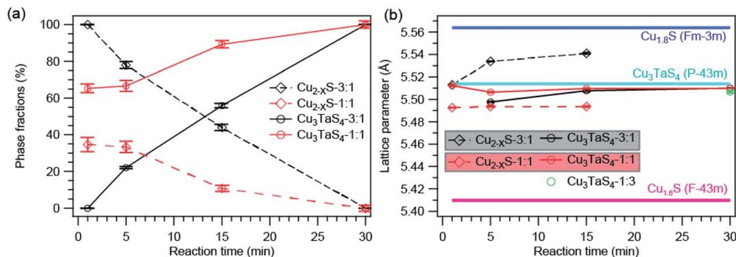
Fig. 3 Analysis from Rietveld refinement profile. (a) Phase fractions of  $\text{Cu}_{2-x}\text{S}$  and  $\text{Cu}_3\text{TaS}_4$  as a function of reaction time. (b) The calculated lattice parameters of  $\text{Cu}_{2-x}\text{S}$  and  $\text{Cu}_3\text{TaS}_4$  compared with standard lattice parameters of  $\text{Cu}_{1.8}\text{S}$ ,  $\text{Cu}_{1.6}\text{S}$ , and  $\text{Cu}_3\text{TaS}_4$ .
