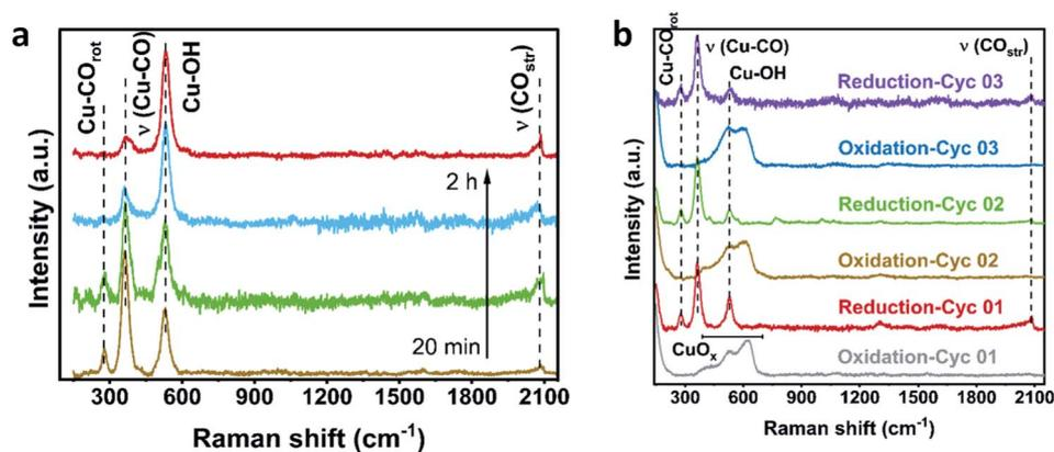
Fig. 4 *In situ* Raman studies on oxidized Cu species of Cu/PTFE. (a) *In situ* SERS of Cu/PTFE conducted at different times of reaction in  $KHCO_3$  electrolyte at a current density of 30  $mA\ cm^{-2}$ . (b) The structure and surface adsorbates during reduction and oxidation cycles at 0.6  $mA\ cm^{-2}$  oxidation current density for 20 s.
