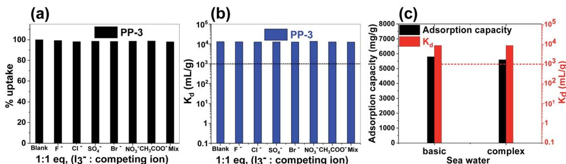
Fig. 7 (a) Uptake percent for  $I_3^-$  anions in the presence of other competing anions, (b) distribution coefficient ( $K_d$ ) graph and (c)  $I_3^-$  adsorption capacity from the basic and complex seawater and the corresponding distribution coefficient value ( $K_d$ ).
