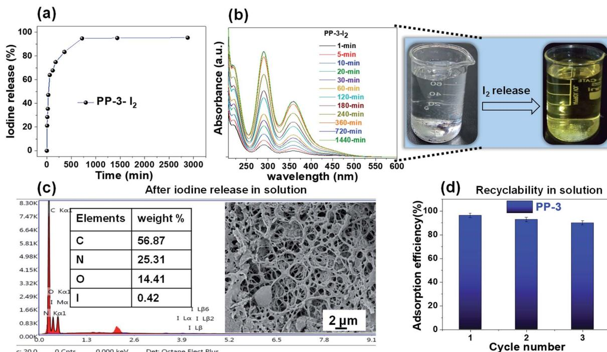
Fig. 9 (a) Iodine release kinetics with heating at 140 °C, (b) UV spectra of rapid iodine release from PP-3-I<sub>2</sub> in methanol (image showing the visual color change for iodine release), and (c and d) EDX analysis of PP-3 after iodine release (FESEM image inset) and reusability of PP-3 for iodine adsorption, respectively in solution.
