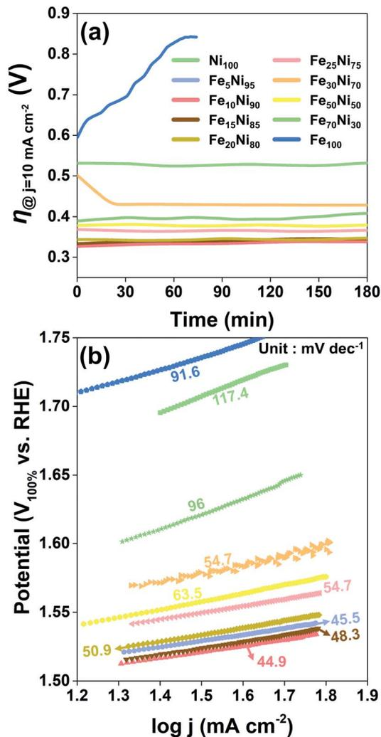
Fig. 3 (a) Chronoamperometry tests conducted at  $10 \text{ mA cm}^{-2}$  vs. RHE at the controlled temperature of  $25 \text{ }^\circ\text{C}$  in  $1 \text{ M KOH}$  for 180 min; and (b) Tafel plots and slopes of  $\text{FeNiO}_x\text{H}_y$  acquired free of  $iR$  drop at a low scan rate of  $5 \text{ mV s}^{-1}$  to suppress capacitive current.
