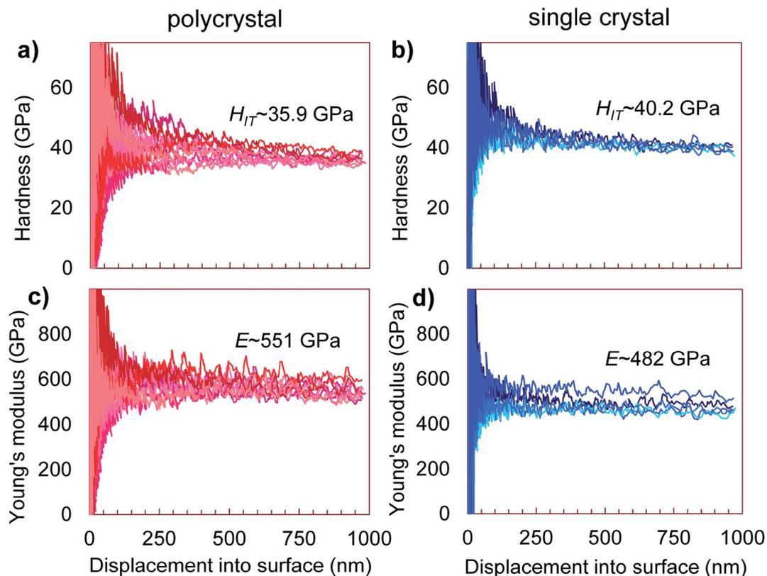
Fig. 5 The nanoindentation hardness,  $H_{IT}$  (a and b), and Young's modulus,  $E$  (c and d) of polycrystals (a and c) and single crystals (b and d) of  $WB_4$  at 295 K. Each plot combines several tests and shows average values.
