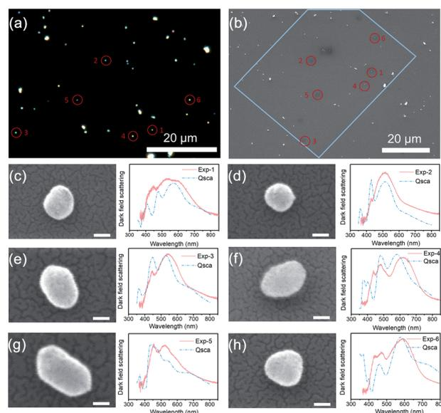
Fig. 2 (a) Optical DFS image of  $\text{TiO}_2$  NPs on the glass substrate. (b) *In situ* SEM image of the  $\text{TiO}_2$  NPs in (a). (c–h) Left panel: zoom-in SEM image for single  $\text{TiO}_2$  NPs numbered 1–6 in (a and b); right panel: corresponding experimental DFS spectra (pink solid lines) and simulated scattering efficiency  $Q_{\text{sca}}$  (blue dashed lines). The scale bar is 100 nm in (c–h).
