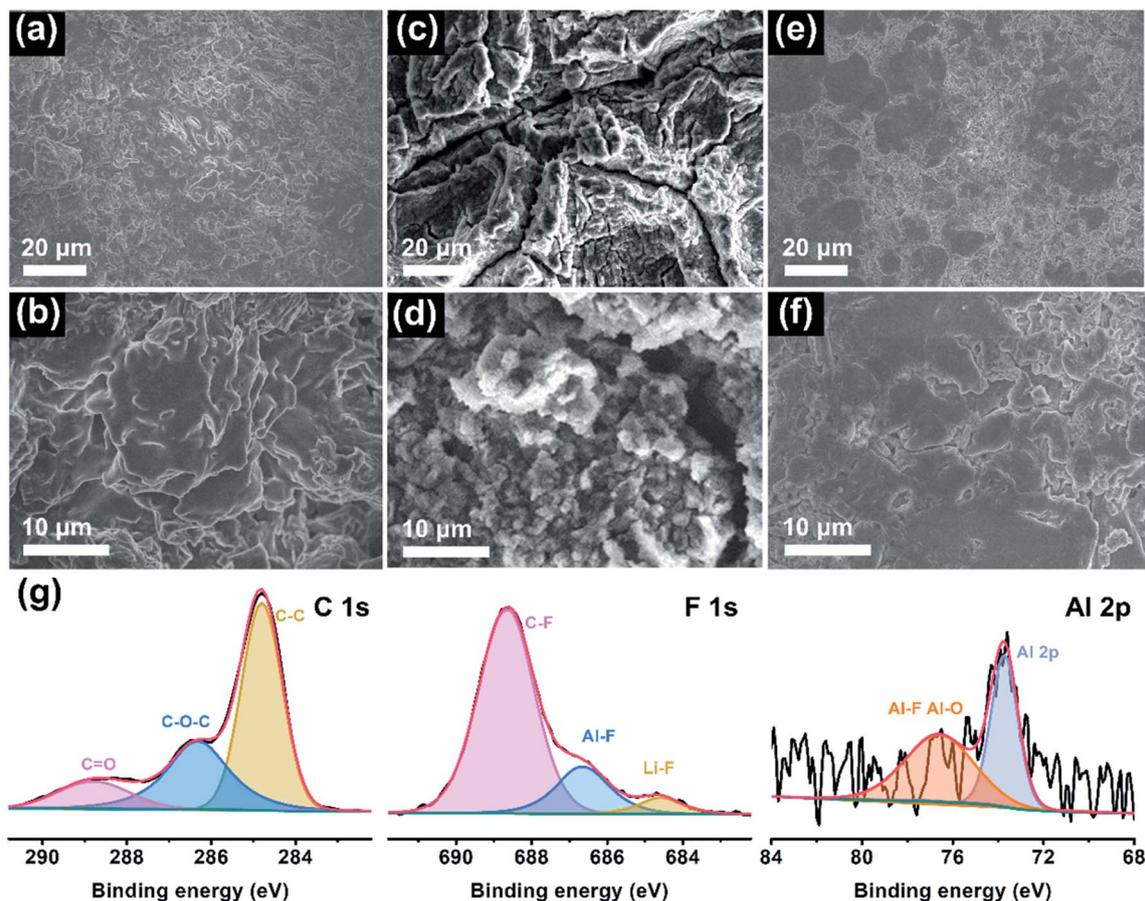
Fig. 4 Interfacial characterizations of the anode surface. SEM images of Li metal after 50 cycles with (a and b) PDOL electrolyte, (c and d) *Ex-situ* PLE and (e and f) *In-situ* PLE. (g) XPS spectra of the cycled Li anode from the symmetric battery using *In-situ* PLE.
