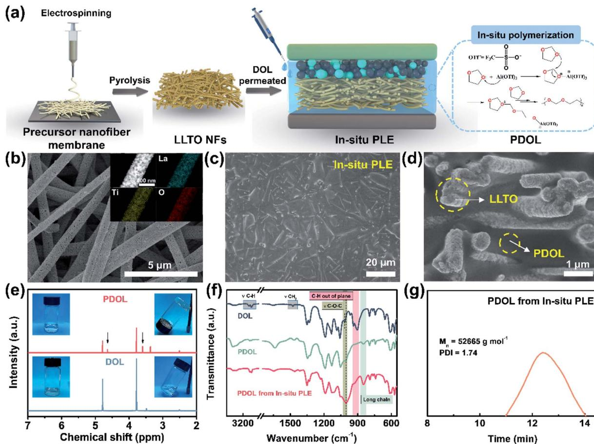
Fig. 1 (a) Schematic illustrating the preparation of the *In-situ* PLE via *in situ* polymerization. (b) Surface morphology of LLTO NFs membrane. The inset shows the EDS mappings of La, Ti, and O elements. SEM images of the *In-situ* PLE: (c) surface, and (d) cross-section. (e)  $^1\text{H}$  NMR spectra of liquid DOL and solid PDOL. The inset depicts the unchanged liquid DOL electrolyte and solidified PDOL electrolyte. (f) FTIR spectra. (g) The average molecular weight of PDOL obtained by GPC.
