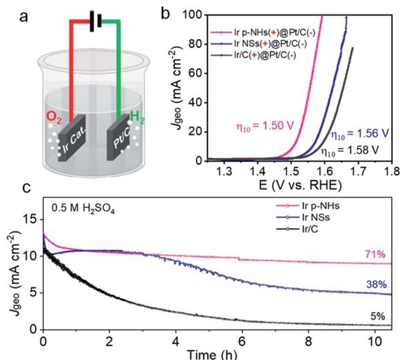
Fig. 4 Initial electrocatalytic overall water splitting performance in 0.5 M  $\text{H}_2\text{SO}_4$ . (a) Scheme of the two-electrode cell electrolyzer using the Ir-based catalyst as the anode and 20% Pt/C as the cathode. (b) Polarization curves of Ir p-NHs, Ir NSs and Ir/C for overall water splitting. (c) Durability test for the three catalysts in a two-electrode configuration.
