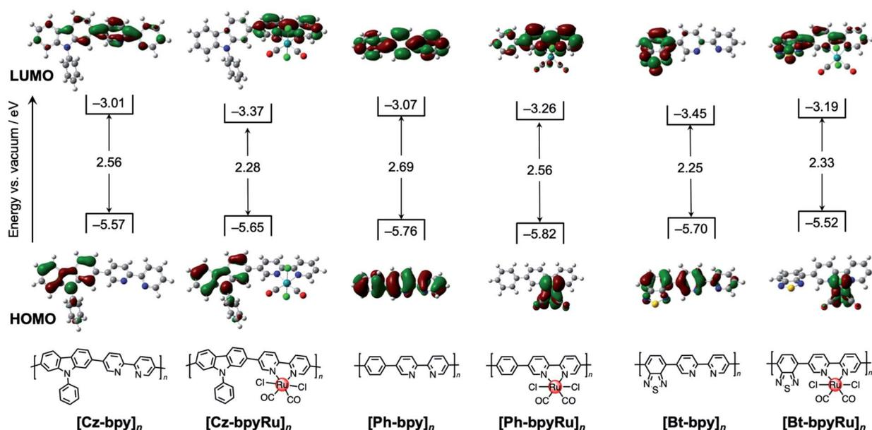
Fig. 2 Experimentally-estimated band positions of [X-bpyM]<sub>n</sub> (X = Cz, Ph, and Bt; M = none and Ru) along with calculated HOMO (lower) and LUMO (upper) distributions of X-bpyM.
