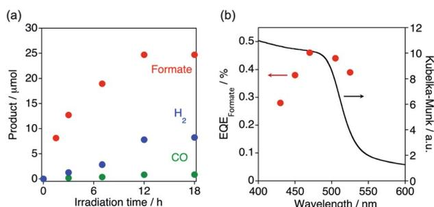
Fig. 5 (a) Time courses of photocatalytic reaction and (b) action spectra of external quantum efficiency of formate formation ( $\text{EQE}_{\text{formate}}$ ) by [Cz-bpyRu]<sub>n</sub> (2 mg) in an MeCN-TEOA (2 mL; 4 : 1 v/v) dispersion under CO<sub>2</sub> atmosphere.
