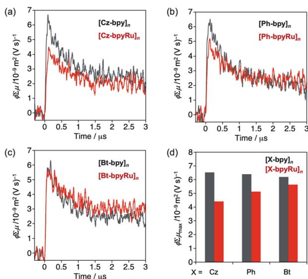
Fig. 3 Transient conductivities of (a)  $[\text{Cz-bpyM}]_n$ , (b)  $[\text{Ph-bpyM}]_n$ , and (c)  $[\text{Bt-bpyM}]_n$  (M = none (grey) or Ru (red)), along with (d) their maximum values ( $\phi\Sigma\mu_{\text{max}}$ ) obtained by photoexcitation at  $\lambda = 355$  nm.
