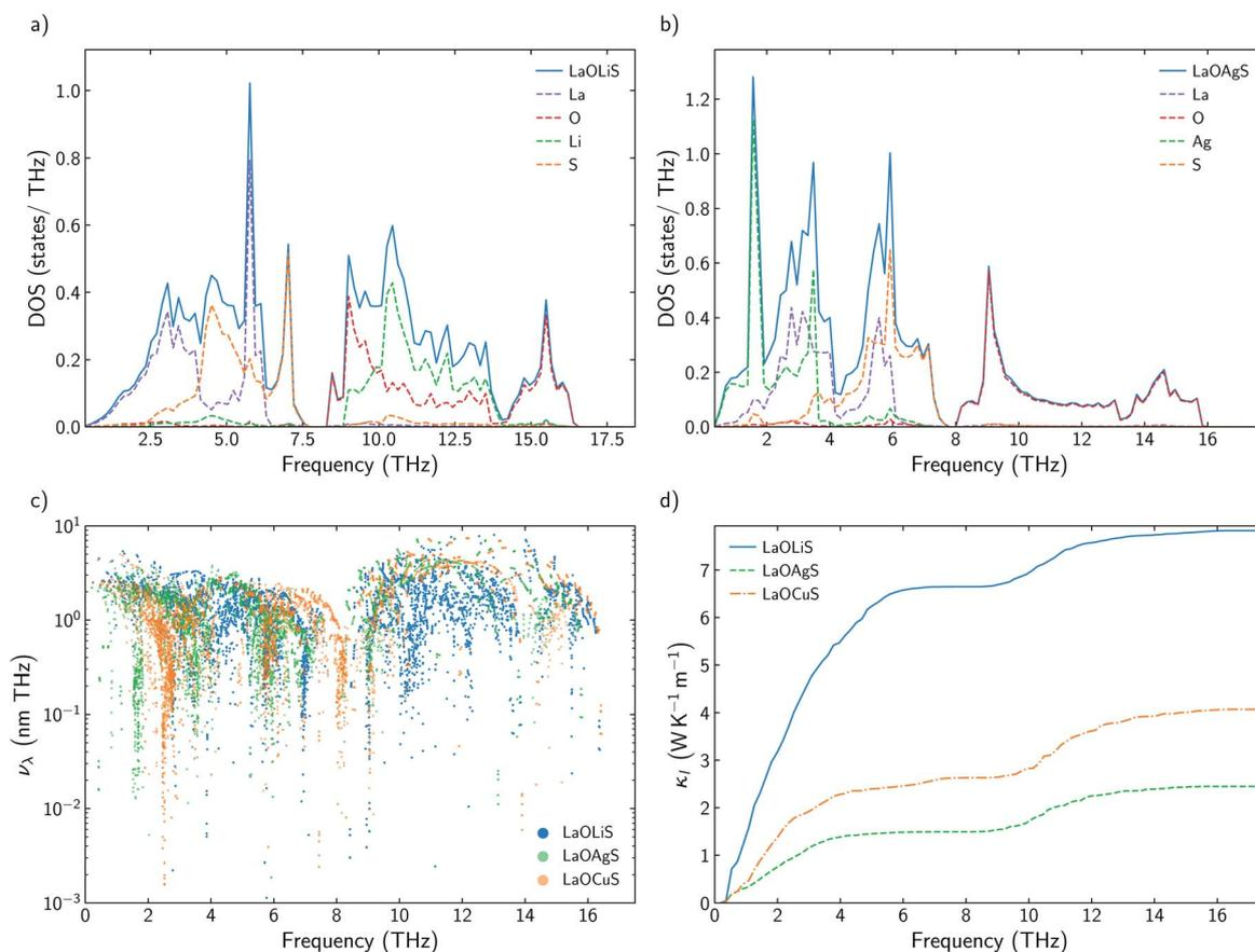
Fig. 5 (a and b) Total and projected phonon density of states, DOS, of LaOLiS and LaOAgS. (c) Group velocities,  $v_g$  for LaOLiS (blue), LaOCuS (green), and BiOCuS (orange). (d) Cumulative  $\kappa_1$  for LaOLiS (blue solid line), BiOAgS (green dashed line) and BiOCuS (orange dashed line).
