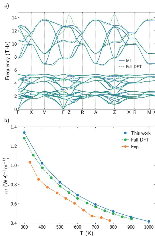
Fig. 1 (a) Comparison of BiOCuSe phonon dispersion curves obtained using the machine-learned force constant potential, ML, *via* HiPhive with those from the full-DFT method *via* Phonopy. (b) Comparison of experimental  $\kappa_1$  (orange)<sup>14</sup> with calculated results using a full-DFT approach (green),<sup>41</sup> and ML-based model (blue) between 300 and 900 K.
