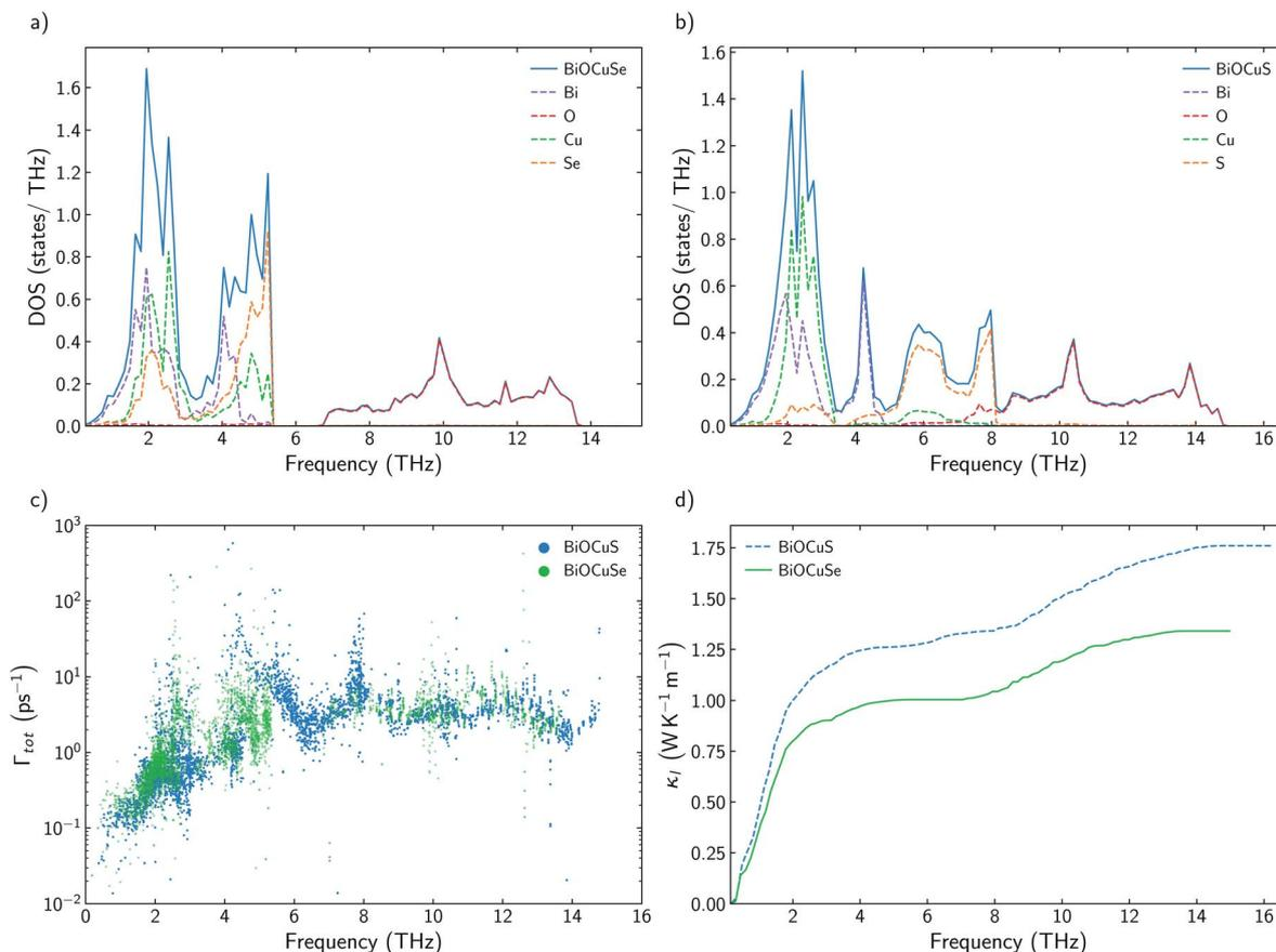
Fig. 2 (a and b) Total and projected phonon density of states, DOS, of BiOCuSe and BiOCuS. (c) Total scattering rates,  $\Gamma_{tot}$  for BiOCuSe (green) and BiOCuS (blue) at 300 K. (d) Cumulative  $\kappa_l$  for BiOCuSe (green solid line) and BiOCuS (blue dashed line) at 300 K.
