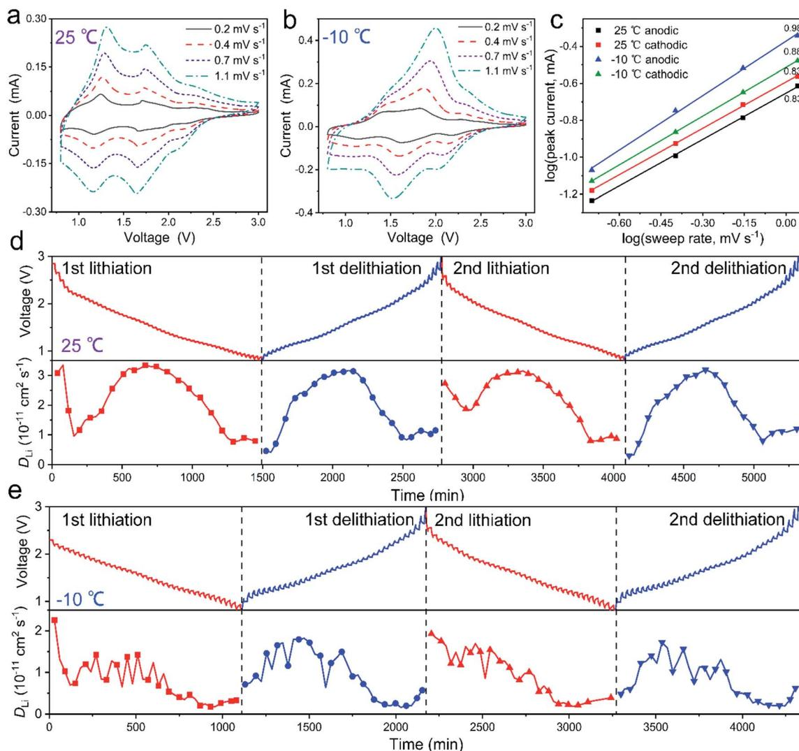
Fig. 5 Electrochemical kinetics of  $\text{Mo}_4\text{Nb}_{26}\text{O}_{77}$  submicron-sized particles. CV profiles of the  $\text{Mo}_4\text{Nb}_{26}\text{O}_{77}/\text{Li}$  half cell at (a) 25 and (b)  $-10$  °C at different sweep rates. (c) Linear relationship between  $\log(\text{current})$  and  $\log(\text{sweep rate})$ . GITT curves and variations in  $\text{Li}^+$  diffusion coefficients (first two cycles) at (d) 25 and (e)  $-10$  °C.
