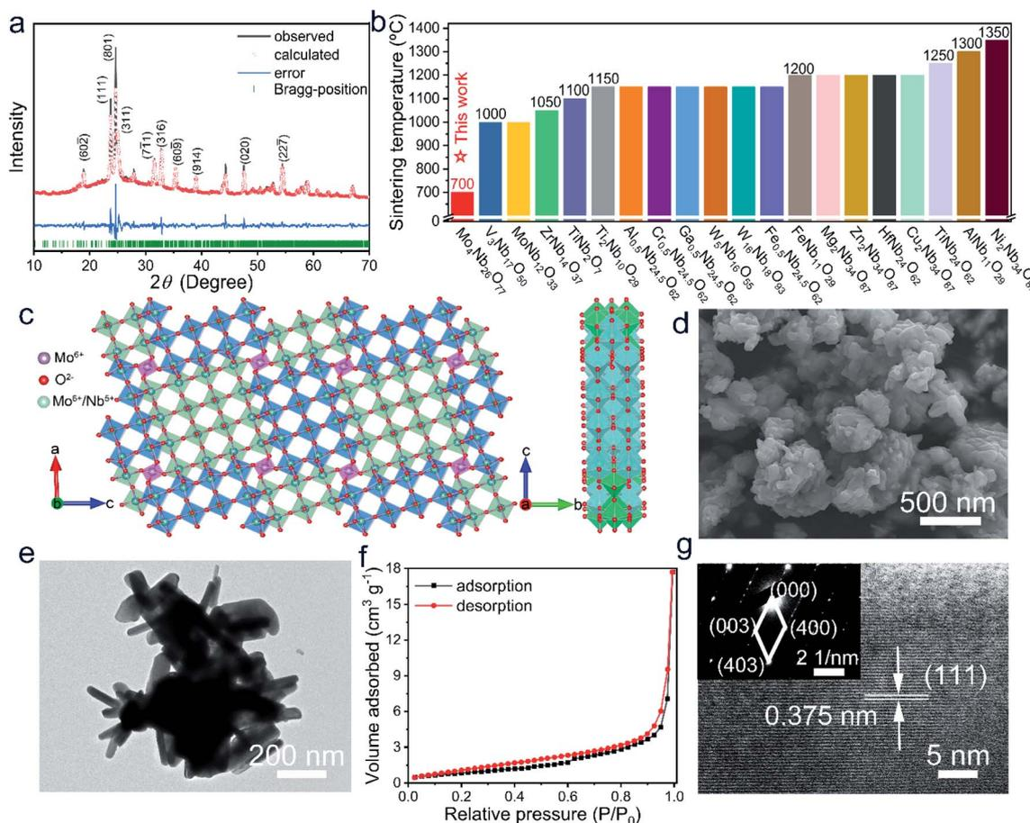
Fig. 1 Physico-chemical characterization studies of  $\text{Mo}_4\text{Nb}_{26}\text{O}_{77}$ . (a) Rietveld-refined XRD pattern. (b) Sintering temperature of  $\text{Mo}_4\text{Nb}_{26}\text{O}_{77}$  from the solid-state reaction compared with other niobates. (c) Crystal structure viewed from different directions. (d) FESEM and (e) TEM images. (f)  $\text{N}_2$  adsorption–desorption isotherms. (g) HRTEM image (inset: SAED pattern).
