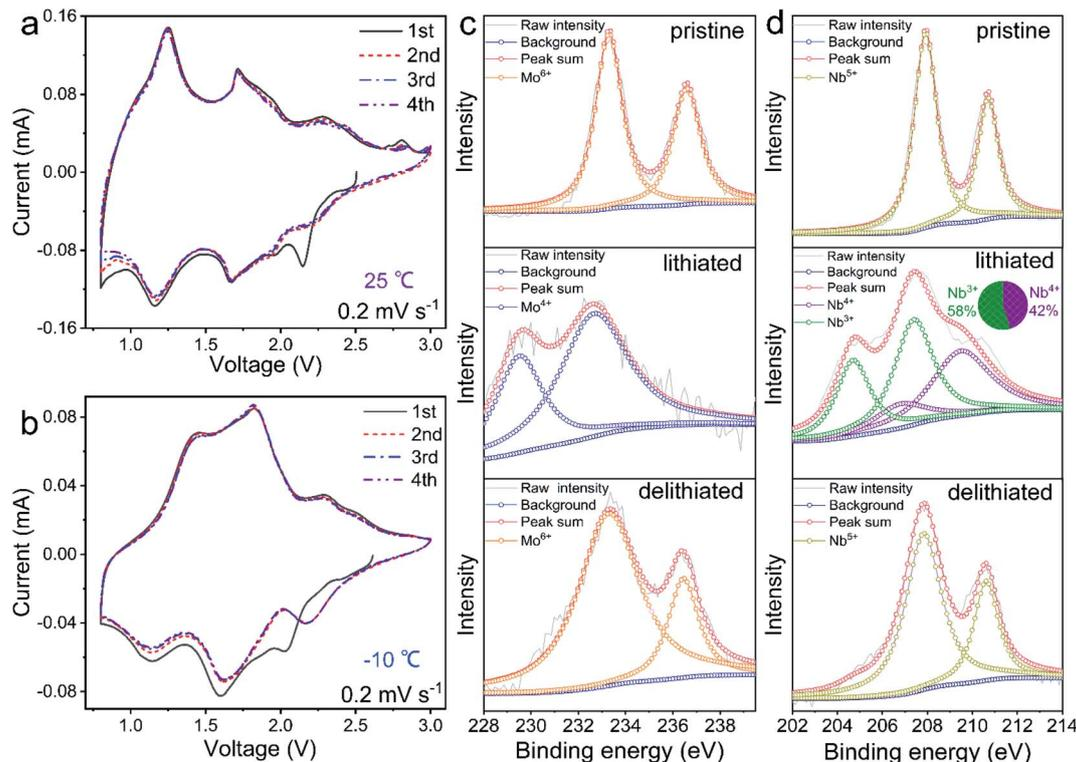
Fig. 4 Redox mechanism of  $\text{Mo}_4\text{Nb}_{26}\text{O}_{77}$  submicron-sized particles. First four-cycle CV profiles of the  $\text{Mo}_4\text{Nb}_{26}\text{O}_{77}/\text{Li}$  half cell at (a) 25 and (b)  $-10$  °C. *Ex situ* (c) Mo-3d and (d) Nb-3d XPS spectra of pristine, lithiated and delithiated  $\text{Mo}_4\text{Nb}_{26}\text{O}_{77}$  samples at 25 °C.
