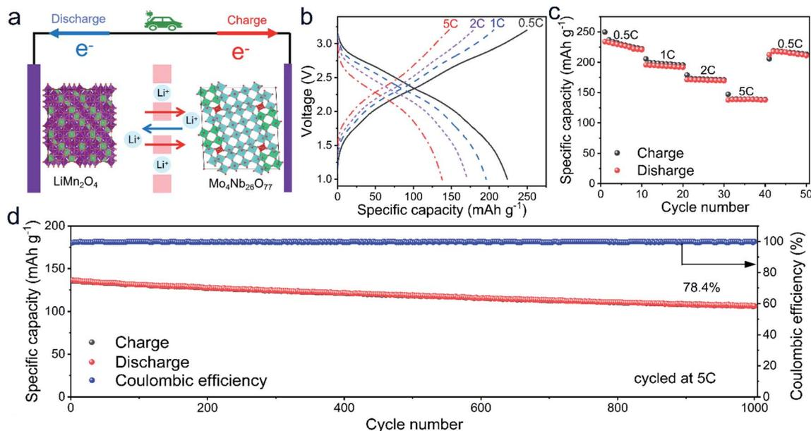
Fig. 3 Electrochemical properties of the  $\text{LiMn}_2\text{O}_4/\text{Mo}_4\text{Nb}_{26}\text{O}_{77}$  full cell. (a) Schematic illustration of a full cell. (b) GCD curves at various current rates. (c) Rate performance. (d) Long-term cyclability over 1000 cycles at 5C.
