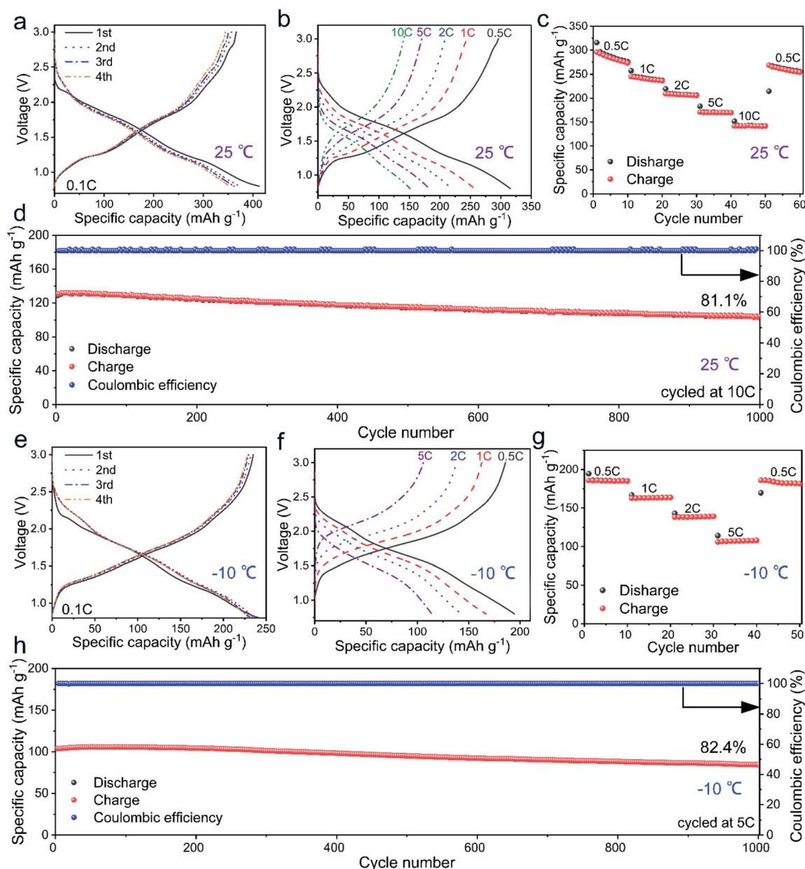
Fig. 2 Electrochemical characterization studies of the  $\text{Mo}_4\text{Nb}_{26}\text{O}_{77}/\text{Li}$  half cell at 25 and  $-10$  °C. (a and e) First four-cycle GCD curves at 0.1C. (b and f) GCD curves at various current rates. (c and g) Rate performance. (d and h) Long-term cyclability over 1000 cycles.
