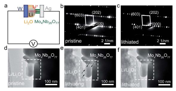
Fig. 7 In situ TEM characterization of Mo<sub>4</sub>Nb<sub>26</sub>O<sub>77</sub> submicron-sized particles. (a) Schematic illustration of the in situ TEM half cell. In situ SAED patterns recorded at (b) pristine and (c) lithiated states. In situ TEM images of Mo<sub>4</sub>Nb<sub>26</sub>O<sub>77</sub> recorded at (d) pristine, (e) lithiating and (f) lithiated states. Significant movement of strain fringes induced by Li<sup>+</sup> insertion is observed within white and dotted rectangles
