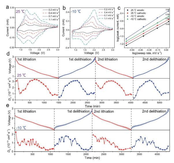
Fig. 5 Electrochemical kinetics of  $Mo_4Nb_{26}O_{77}$  submicron-sized particles. CV profiles of the  $Mo_4Nb_{26}O_{77}$ /Li half cell at (a) 25 and (b) -10 °C at different sweep rates. (c) Linear relationship between log(current) and log(sweep rate). GITT curves and variations in Li<sup>+</sup> diffusion coefficients (first two cycles) at (d) 25 and (e) -10 °C.
