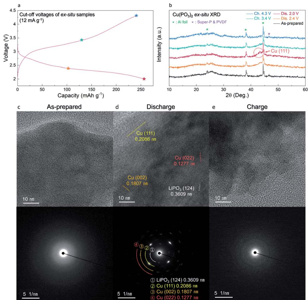
Fig. 5 (a) Cut-off voltage points of the *ex situ* samples on the charge/discharge curve of A-CPO/C. (b) *Ex situ* XRD patterns of A-CPO/C. HRTEM images with SAED patterns of (c) as-prepared, (d) discharged, and (e) charged A-CPO/C.
