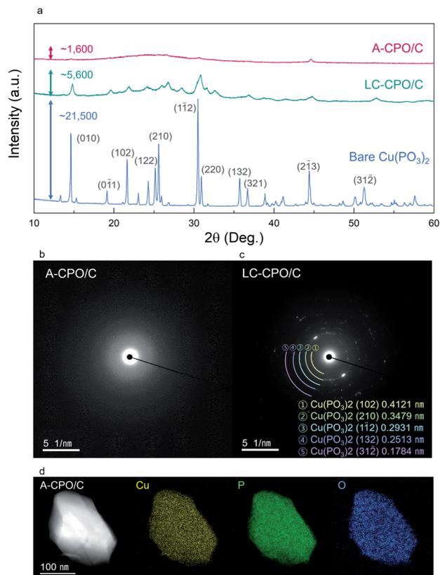
Fig. 2 (a) Comparing XRD patterns and the maximum intensities of bare  $\text{Cu}(\text{PO}_3)_2$ , LC-CPO/C and A-CPO/C. TEM SAED patterns of (b) A-CPO/C, (c) LC-CPO/C, (d) EDS elemental mapping (Cu: yellow, P: green, O: blue) of A-CPO/C.
