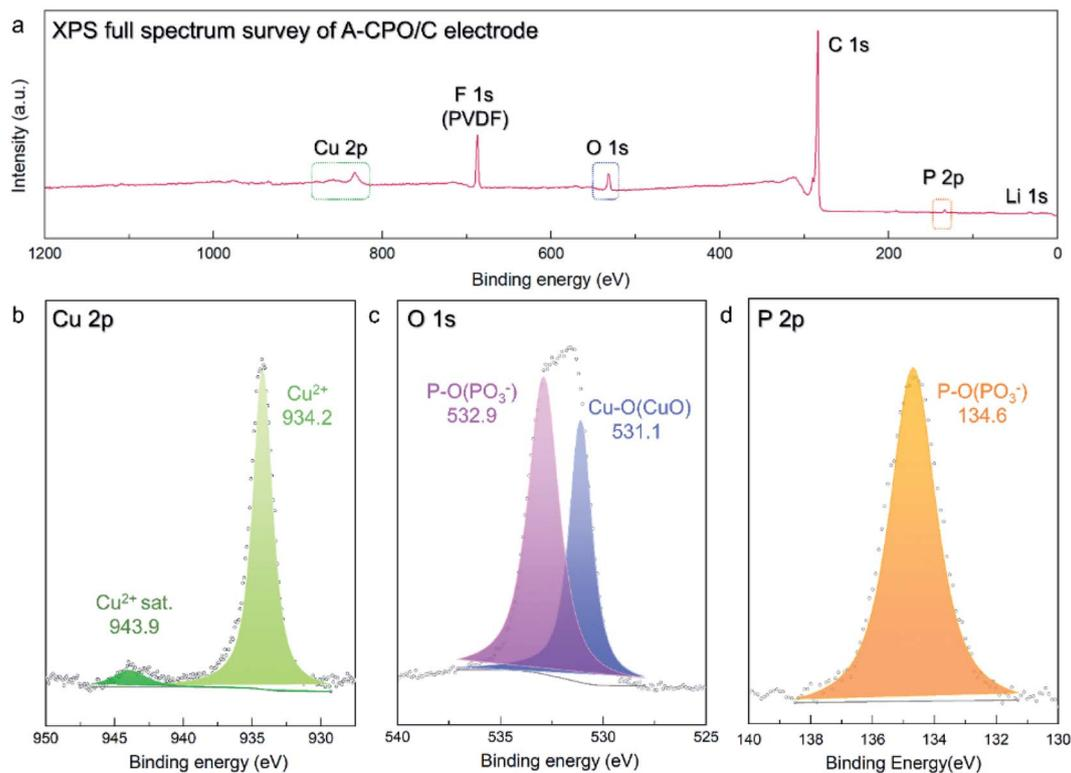
Fig. 3 XPS spectra of A-CPO/C: (a) XPS full spectrum survey, (b) Cu 2p, (c) O 1s, and (d) P 2p.
