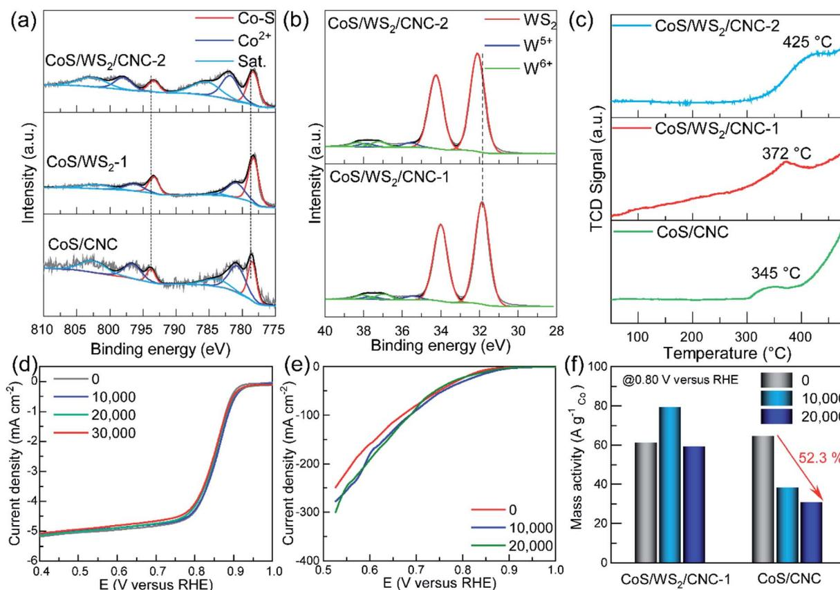
Fig. 3 High-resolution (a) Co 2p and (b) W 4f XPS spectra, and (c) O<sub>2</sub>-TPD profiles of CoS/CNC, CoS/WS<sub>2</sub>/CNC-1, and CoS/WS<sub>2</sub>/CNC-2 catalysts. The polarization curves of CoS/WS<sub>2</sub>/CNC-1 catalyst measured in the (d) RDE and (e) GDE setups during the ADT process, and (f) mass activity ( $J_{\text{mass}}$ ) at  $0.80 \text{ V}$  versus RHE tested in the GDE configuration.
