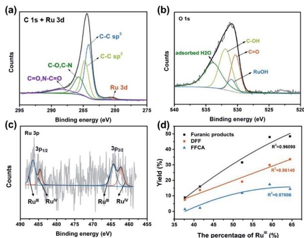
Fig. 8 The high resolution (a) C 1s + Ru 3d, (b) O 1s and (c) Ru 3p XPS spectra of Ru<sub>4</sub>/PEI-rGO upon electrolysis for 6 h at 0.94 V at pH = 6. (d) The plots of the yields of furanic products *versus* the percentage of the Ru<sup>III</sup> species.
