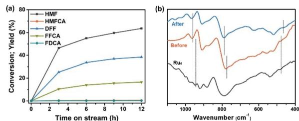
Fig. 9 (a) The long-term bulk electrolysis of Ru<sub>4</sub>/PEI-rGO at an applied voltage of 0.94 V in pH 6 electrolyte solution. (b) FT-IR spectra of Ru<sub>4</sub> and Ru<sub>4</sub>/PEI-rGO before and after long-term electrolysis.
