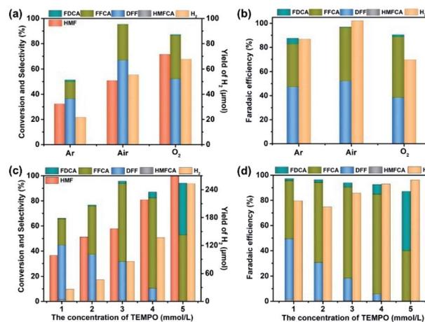
Fig. 6 The effects of the reaction atmosphere (a and b) and concentration of TEMPO (c and d) on the electrocatalytic activities of  $\text{Ru}_4/\text{PEI-rGO}$ .
