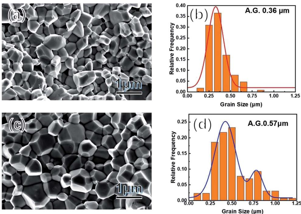
Fig. 3 (a and c) SEM images of freshly fractured surfaces of  $\text{Co}_{0.94}\text{Ni}_{0.06}\text{SbS}$  and  $\text{Co}_{0.94}\text{Ni}_{0.06}\text{SbS}_{0.96}\text{Te}_{0.04}$ , respectively; (b and d) their corresponding grain-size distribution analysis.
