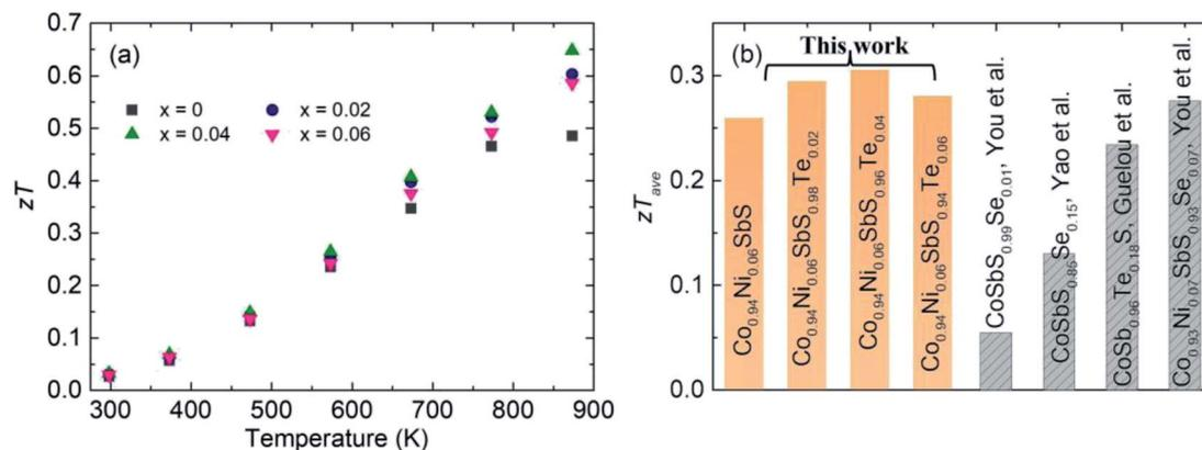
Fig. 6  $zT$  value of the  $\text{Co}_{0.94}\text{Ni}_{0.06}\text{SbS}_{1-x}\text{Te}_x$  samples ( $x = 0, 0.02, 0.04$ , and  $0.06$ ). (a) Temperature-dependent  $zT$  values and (b) comparison of the  $\text{Co}_{0.94}\text{Ni}_{0.06}\text{SbS}_{1-x}\text{Te}_x$  samples with other reported CoSbS samples prepared by Hou *et al.*, Yao *et al.*, and Guelou *et al.*
