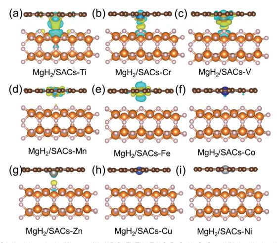
Fig. 5 (a–i) Calculated charge density differences of MgH<sub>2</sub>/SACs–TM (TM = Ti, V, Cr, Zn, Cu, Mn, Co, Fe, and Ni) induced by the addition of SACs. The yellow and blue isosurfaces indicate electron accumulation and loss, respectively. All the results are plotted with an isovalue of 0.001 e  $\mathring{A}^{-3}$ . White, orange, brown, and gray spheres represent H, Mg, C, and N, respectively.
