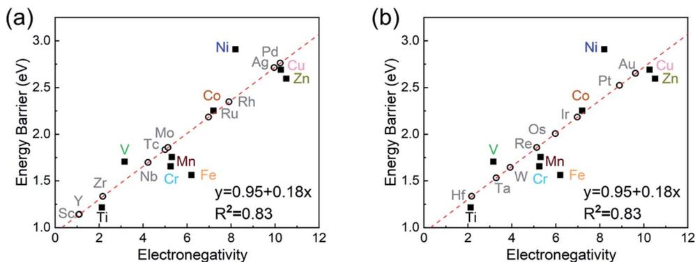
Fig. 8 Prediction of dehydrogenation energy barriers at  $\text{MgH}_2/\text{SACs-TM}$  based on the linear correlation of dehydrogenation barrier vs. electronegativity. The empty and solid dots represent the predicted and DFT-calculated values, respectively. In (a), the elements consist of Sc and 5d TMs: TM = Sc, Y, Zr, Nb, Mo, Tc, Ru, Rh, Pd, and Ag. In (b), the elements consist of 4d TMs: TM = Hf, Ta, W, Re, Os, Ir, Pt, and Au.
