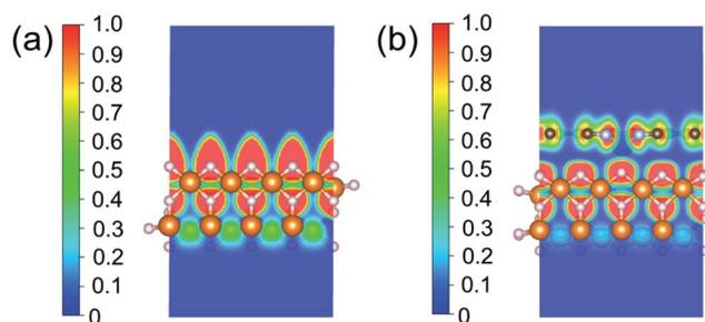
Fig. 4 ELFs of (a) MgH<sub>2</sub> and (b) MgH<sub>2</sub>/SACs–Ti. The section is the O10 plane of the H atom nearest to the metal atom. In the color bars, 1 represents a fully localized state, 0.5 represents a uniform electronic gas state, and 0 represents a fully nonlocalized state. The ELF results of other MgH<sub>2</sub>/SAC systems are shown in Fig. S4.†
