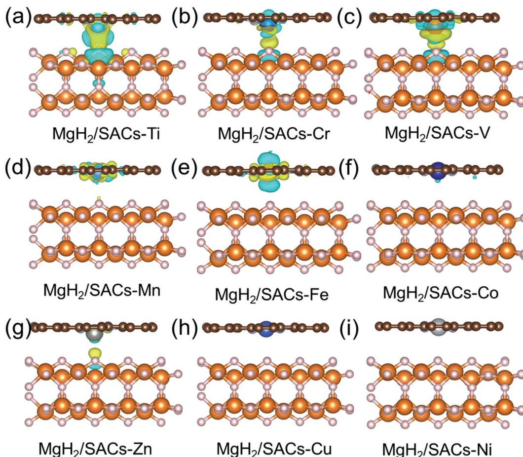
Fig. 5 (a–i) Calculated charge density differences of  $\text{MgH}_2/\text{SACs-TM}$  (TM = Ti, V, Cr, Zn, Cu, Mn, Co, Fe, and Ni) induced by the addition of SACs. The yellow and blue isosurfaces indicate electron accumulation and loss, respectively. All the results are plotted with an isovalue of  $0.001 \text{ e } \text{\AA}^{-3}$ . White, orange, brown, and gray spheres represent H, Mg, C, and N, respectively.
