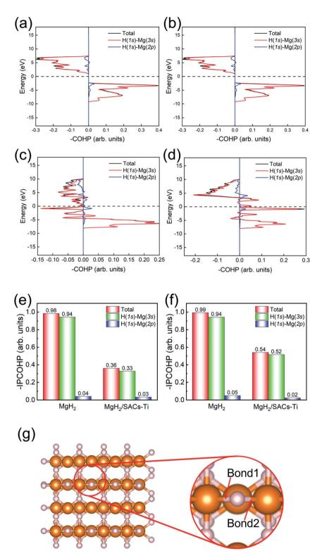
Fig. 7 (a and b) COHP analysis of the Mg-H bond 1 and bond 2 in MgH<sub>2</sub>. (c and d) COHP analysis of the Mg-H bond 1 and bond 2 in MgH<sub>2</sub>/SACs-Ti. (e and f) Comparison of the integral values of Mg-H bond 1 and bond 2 between MgH $_2$  and MgH $_2$ /SACs-Ti in the systems. (g) Illustrations of the bond 1 and bond 2 in MgH<sub>2</sub>. White and orange spheres represent H and Mg, respectively.
