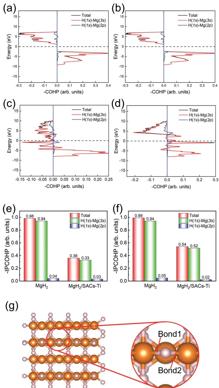
Fig. 7 (a and b) COHP analysis of the Mg–H bond 1 and bond 2 in MgH<sub>2</sub>. (c and d) COHP analysis of the Mg–H bond 1 and bond 2 in MgH<sub>2</sub>/SACs–Ti. (e and f) Comparison of the integral values of Mg–H bond 1 and bond 2 between MgH<sub>2</sub> and MgH<sub>2</sub>/SACs–Ti in the systems. (g) Illustrations of the bond 1 and bond 2 in MgH<sub>2</sub>. White and orange spheres represent H and Mg, respectively.
