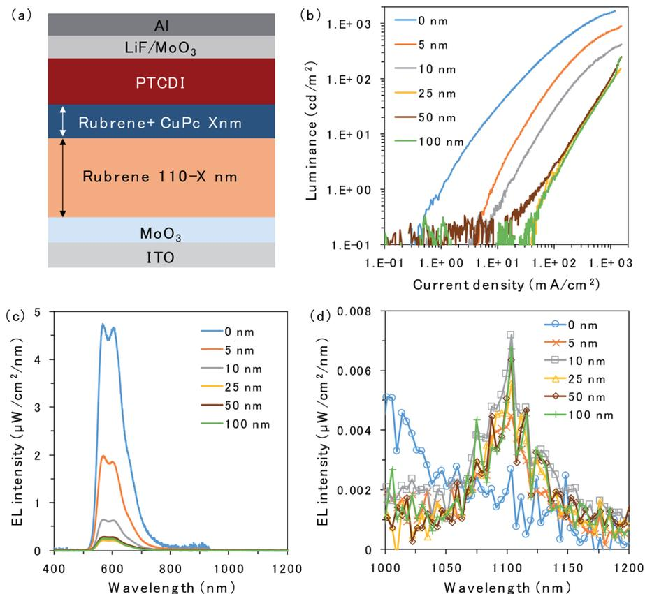
Fig. 2 (a) Schematic of the device with the CuPc-doped rubrene layer at the D/A interface. (b)  $L$ - $J$  curves and (c and d) EL emission spectra with a constant current flow ( $1000 \text{ mA cm}^{-2}$ ) for the devices with 0 nm (blue), 5 nm (orange), 10 nm (grey), 25 nm (yellow), 50 nm (brown), and 100 nm (green) of CuPc-doped rubrene layers at the D/A interface.
