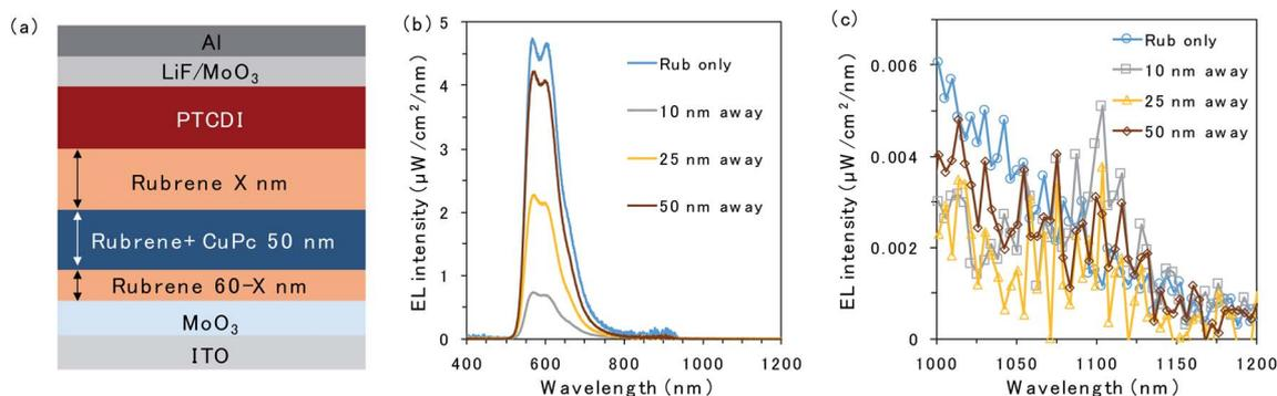
Fig. 3 (a) Schematic of the device with 50 nm of a CuPc-doped rubrene layer away from the D/A interface. (b and c) EL emission spectra with a constant current flow ( $1000 \text{ mA cm}^{-2}$ ) for the devices without CuPc doping (blue) and with 50 nm of a CuPc-doped rubrene layer away from the D/A interface. The thicknesses of rubrene interlayers at the D/A interface are 10 nm (grey), 25 nm (yellow), and 50 nm (brown).
