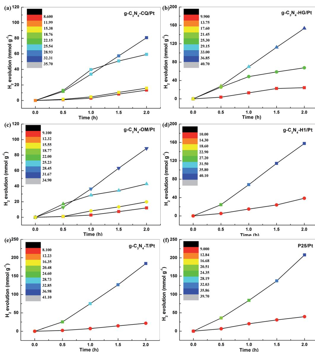
Fig. 3 The general phenomenon for STAP  $H_2$  evolution kinetics. The  $H_2$  evolution yield correlated with system temperature elevation at a variable time under simulated solar light irradiation for the photocatalyst of (a)  $g-C_3N_4$ -CQ/Pt, (b)  $g-C_3N_4$ -HG/Pt, (c)  $g-C_3N_4$ -OM/Pt, (d)  $g-C_3N_4$ -H1/Pt, (e)  $g-C_3N_4$ -T/Pt, (f) P25 ( $TiO_2$ )/Pt. Inset: color scale bar representing system temperature elevation. Photocatalyst loading, 10 mg.
