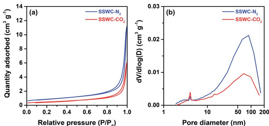
Fig. 4 (a) N<sub>2</sub> adsorption–desorption isotherm; (b) pore size distribution under N<sub>2</sub> physisorption for SSWC-N<sub>2</sub> and SSWC-CO<sub>2</sub>.
