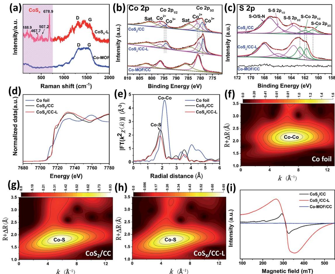
Fig. 2 (a) Raman spectra and high-resolution XPS spectra of the Co 2p (b), S 2p (c) for Co-MOF/CC, CoS<sub>x</sub>/CC-L and CoS<sub>2</sub>/CC. (d) Normalized Co K-edge XANES spectra and (e) Fourier transform of  $k^2$ -weighted Co EXAFS spectra of Co foil, CoS<sub>x</sub>/CC-L and CoS<sub>2</sub>/CC. (f–h) WT-EXAFS spectra of the Co foil, CoS<sub>2</sub>/CC and CoS<sub>x</sub>/CC-L. (i) EPR spectra of Co-MOF/CC, CoS<sub>x</sub>/CC-L and CoS<sub>2</sub>/CC.
