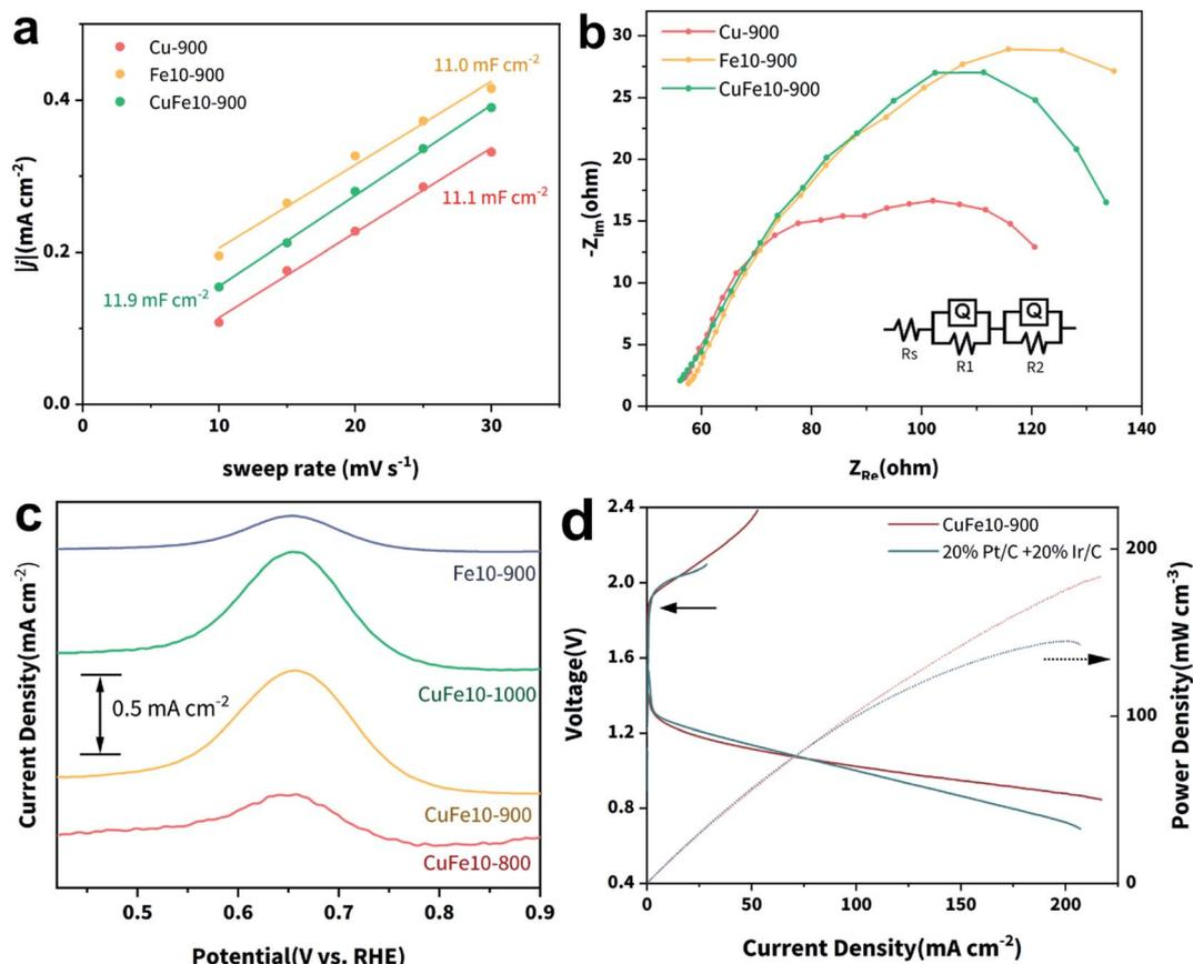
Fig. 4 (a)  $C_{dl}$  fitting plots of Cu-900, Fe10-900 and CuFe10-900, (b) Nyquist plots of the three samples and equivalent circuit, (c) SWV curves of the four SACs and (d) charge–discharge and power density curves of CuFe10-900 and Pt/C for the Zn–air battery.
