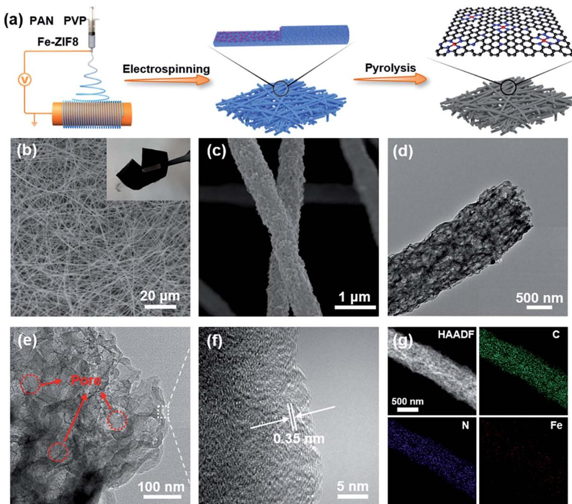
Fig. 1 (a) Schematic illustration of the preparation process of FeSA-PCNF. (b) and (c) SEM images of FeSA-PCNF. The inset of (b) shows the photograph of self-standing and flexible FeSA-PCNF. (d) and (e) TEM images of FeSA-PCNF. (f) HRTEM image of FeSA-PCNF. (g) Elemental mapping images of FeSA-PCNF.
